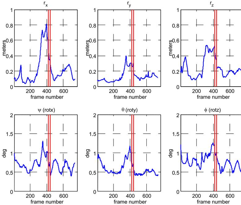
Figure 3.11: Camera location estimate covariance along the sequence. The 95% confidence regions for each of the 6 d.o.f of camera motion are plotted. Note that errors are expressed in a reference local to the camera. The vertical solid lines indicate the loop closing frames #417 and #441.
