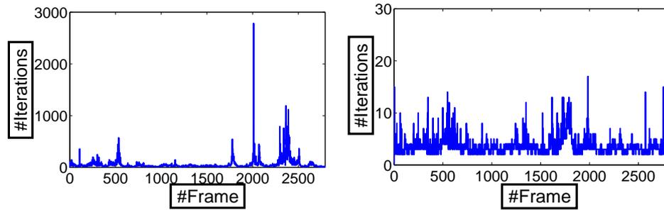
(a) Number of iterations along the sequence for 5-point RANSAC.
