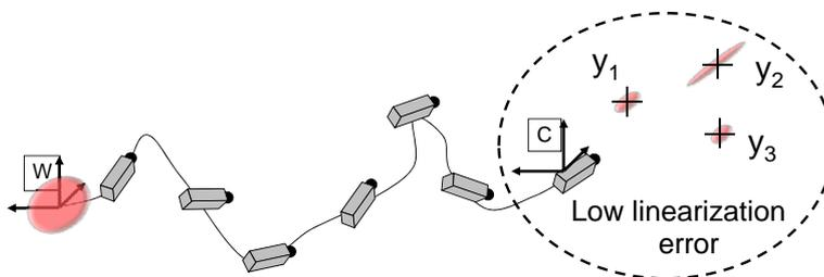
(b) Camera-centered EKF estimation. The camera location uncertainty is close to zero, as the reference is always attached to it. Uncertainties for features in its vicinity  $y_i$  will be also kept low, so measurement model linearization errors will be kept small for the whole estimation.
