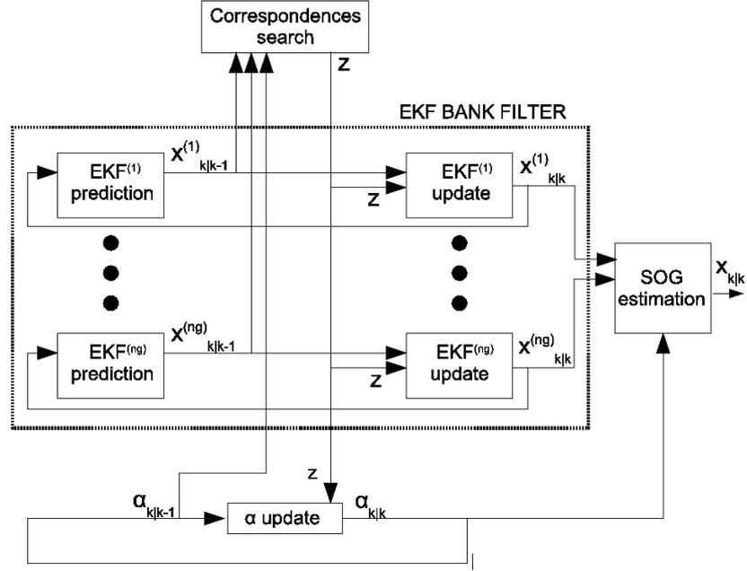
Figure 6.1: Scheme of the Sum of Gaussians (SOG) filter
