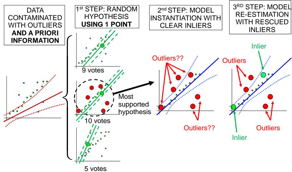
Figure 4.2: 1-Point RANSAC steps for the simple 2D line estimation example: As a key difference from standard RANSAC, the algorithm assumes that an a priori probability distribution over the model parameters is known in advance. This prior knowledge allows us to compute the random hypotheses using only 1 data point, hence reducing the number of hypotheses and the computational cost. The remaining steps do not vary with respect to standard RANSAC in Figure 4.1
