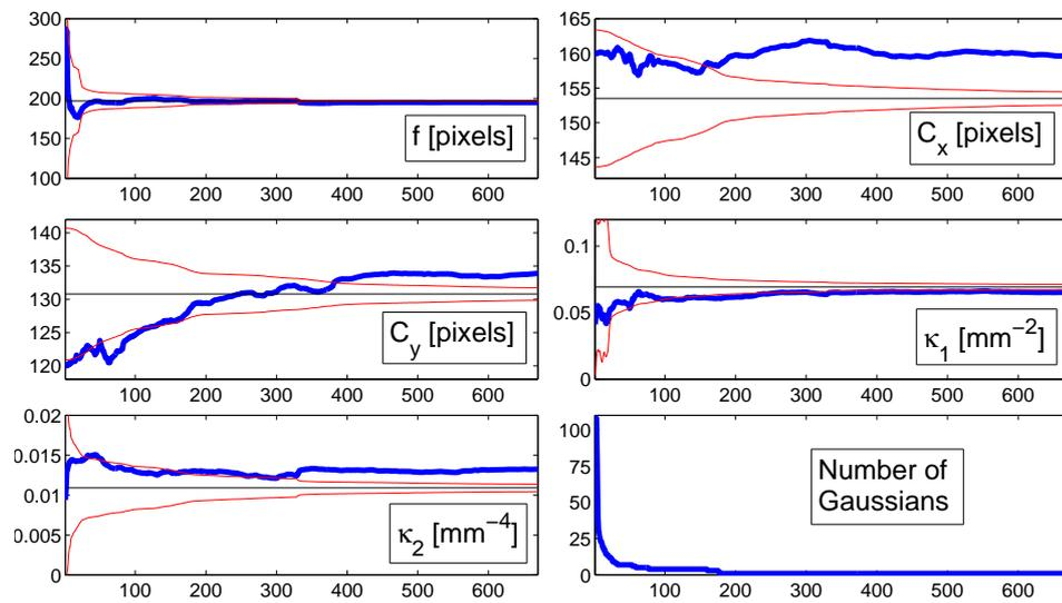
Figure 6.7: Estimated calibration parameters over the loop closing sequence. Thick blue line is the estimated value, the horizontal black line is the offline calibration value and the red thin lines represent the 99% uncertainty region.
