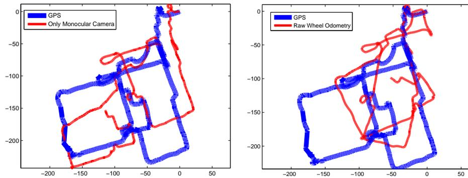
(a) Pure monocular estimation (thin red) tracking 25 features and GPS trajectory (thick blue). Large errors appear caused by scale drift, which is unobservable by a monocular camera.
