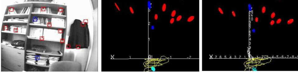
Figure F1: Left: sample. Centre: EKF SLAM estimation result  $\rho_0 = 0.5m^{-1}$ . Right: EKF SLAM estimation result  $\rho_0 = 0.1m^{-1}$ . The uncertainty for the features is plotted in red and blue, the camera uncertainty in cyan and the camera trajectory in yellow.
