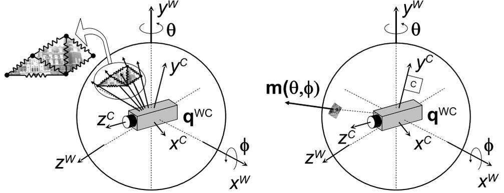
Figure 2.1: Left, An elastic textured triangular mesh is built over a map of scene directions over the unit sphere. Right a scene feature,  $y_i^W$ , stamped with its texture patch.
