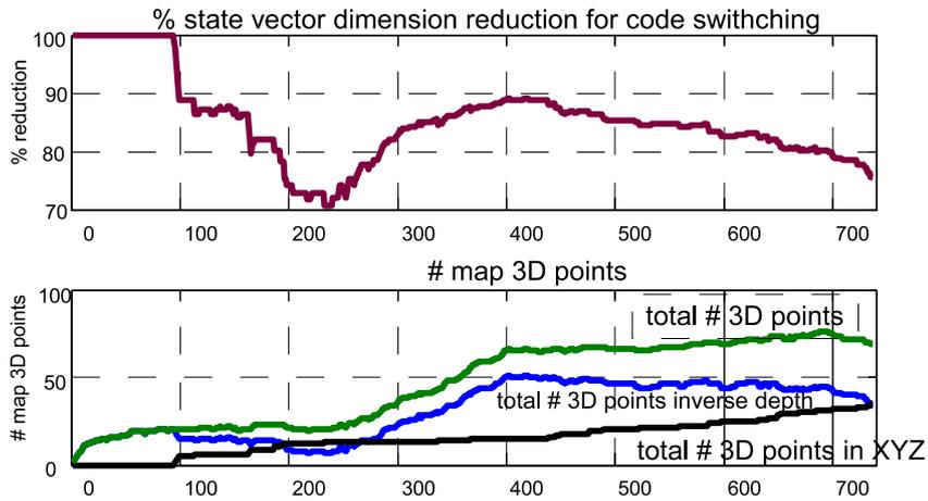
Figure 3.14: Parametrization switching on a real sequence (section 3.8.5): state vector size history. Top: percentage reduction in state dimension when using switching compared with keeping all points in inverse depth. Bottom: total number of points in the map, showing the number of points in inverse depth and the number of points in XYZ.
