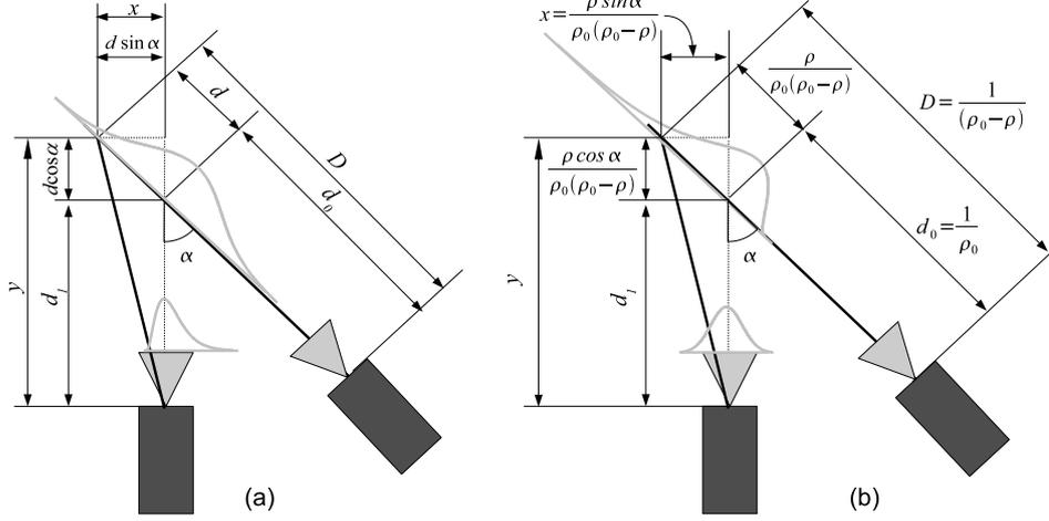
Figure 3.3: Uncertainty propagation from the scene point to the image. (a) XYZ coding. (b) Inverse depth coding.
