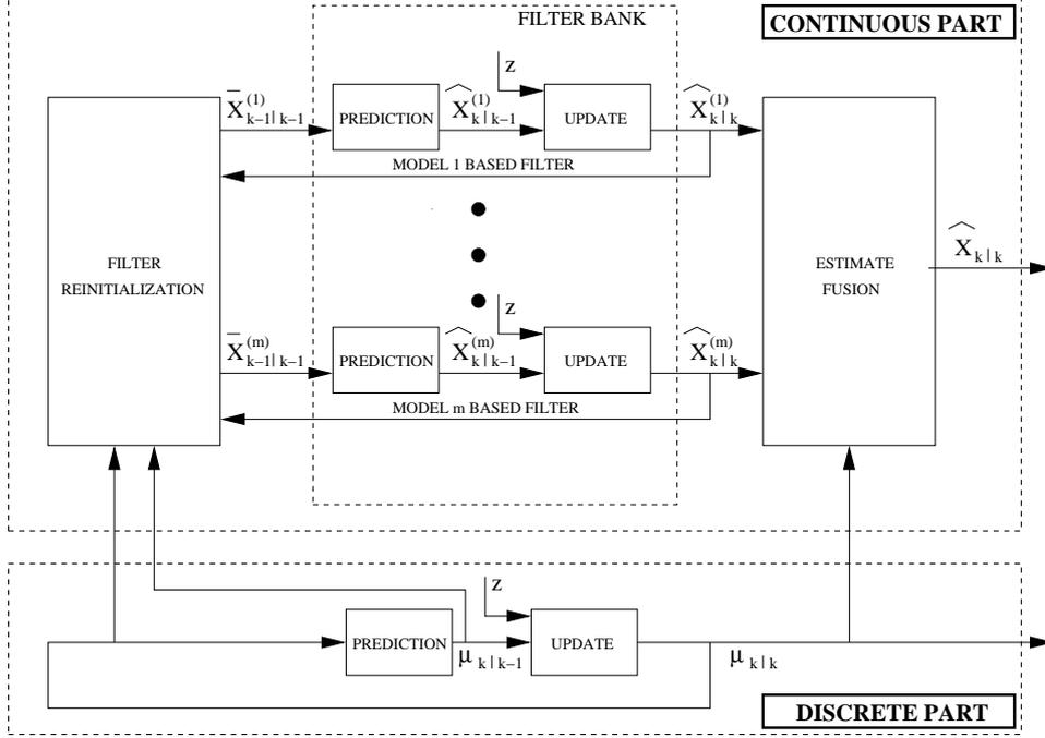
Figure 5.1: Interacting Multiple Model algorithm scheme
