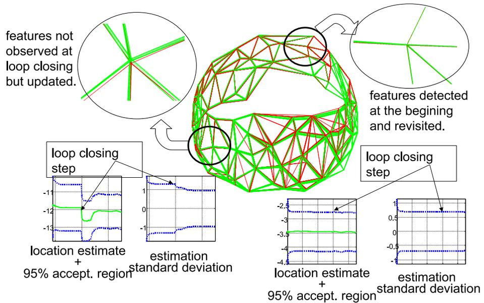
Figure 2.7: Superimposed meshes for 90 frames before loop closure (red) and 90 frames after loop closure (green). The part of the mesh opposite the loop closure is magnified at the left of the figure. The first features detected in the map are magnified at the right of the figure. We also show the camera elevation estimation history along with its standard deviation; notice the uncertainty reduction at loop closure.
