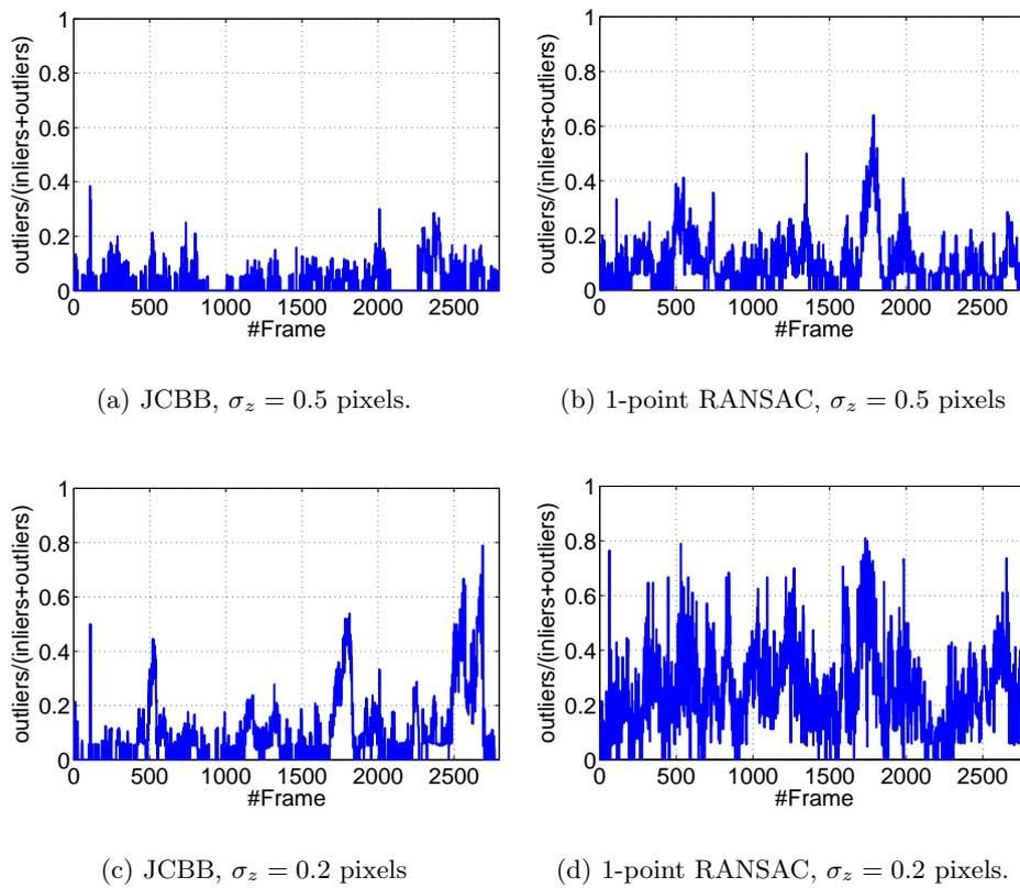
Figure 4.8: Spurious match rate for JCBB and RANSAC when measurement noise standard deviation  $\sigma_z$  is reduced to 0.2 pixels. It can be observed that reducing the measurement noise makes both techniques stricter, but 1-point RANSAC remains more discriminative.
