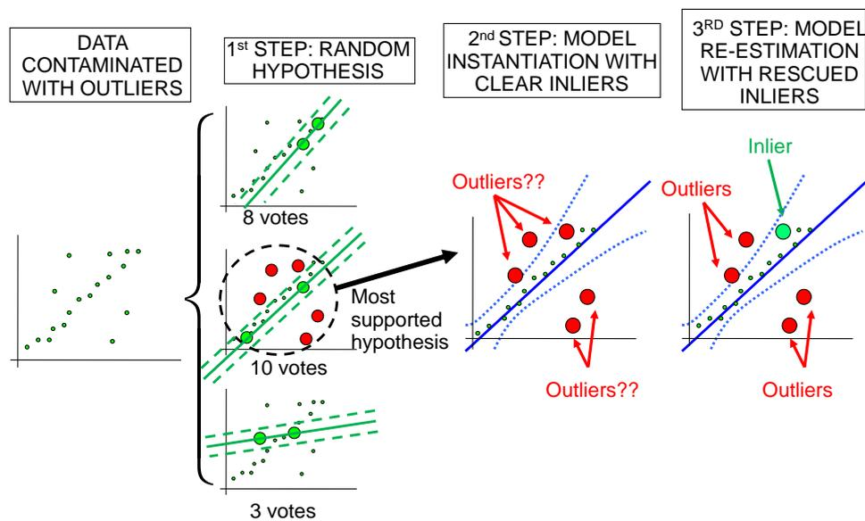
Figure 4.1: RANSAC steps for the simple 2D line estimation example: First, random hypotheses are generated from data samples of size two, the minimum to define a line. The most supported one is selected, and data voting for this hypothesis is considered inlier. Model parameters are estimated from those clear inliers in a second step. Finally, the remaining data points consistent with this latest model are rescued and the model is re-estimated again.
