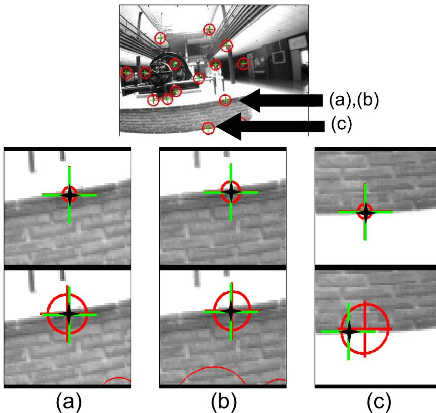
Figure 5.5: (a), IMM (top) and single-model (bottom) feature search ellipse when the camera is rotating. (b), the same feature IMM and single-model search regions when the camera begins to translate. (c), mismatch in the single-model case caused by an unnecessary large ellipse that does not occur in the IMM estimation. Several mismatches like this one in the highly repetitive texture of the brick wall eventually may cause full tracking failure.
