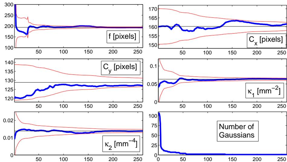
Figure 6.5: Estimated calibration parameters over the computer room sequence. Thick blue line is the estimated value, the horizontal black line is the offline calibration value and the red thin lines represent the 99% uncertainty region.
