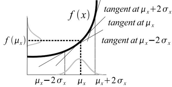
Figure 3.2: The first derivative variation in  $[\mu_x - 2\sigma_x, \mu_x + 2\sigma_x]$  codes the departure from Gaussianity in the propagation of the uncertain variable through a function.
