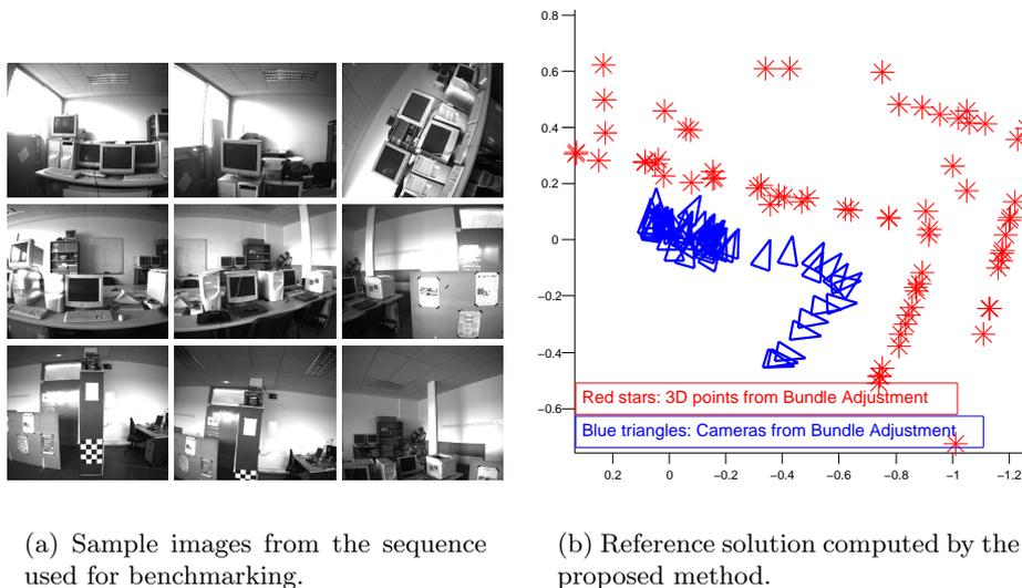
Figure 4.4: Images extracted from the sequence used in the experiments and reference camera positions extracted.
