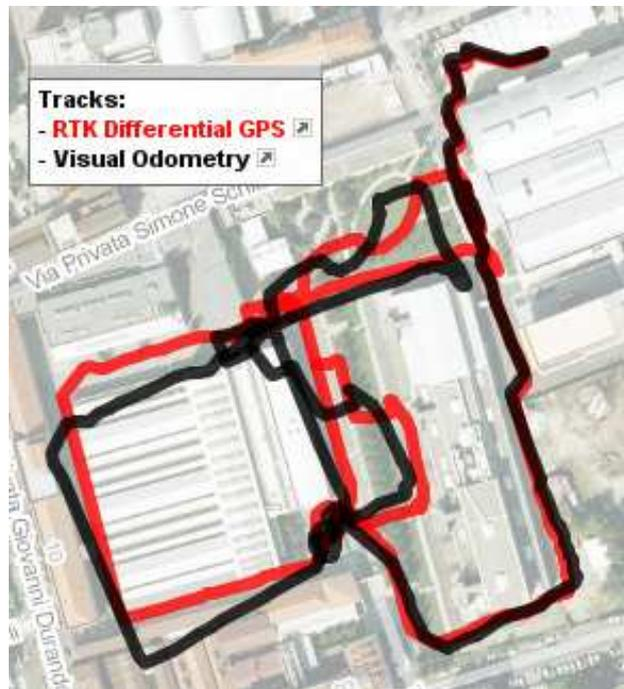
Figure 4.13: Visual odometry results compared against RTK GPS over a Google Maps plot.
