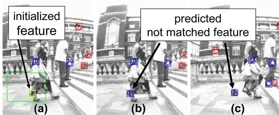
Figure 2.8: (a) Feature initialized on a moving object. (b) after 1 and (c) 10 frames, the feature is no longer matched because it is outside its acceptance region. Eventually this non matching feature is deleted from the map.
