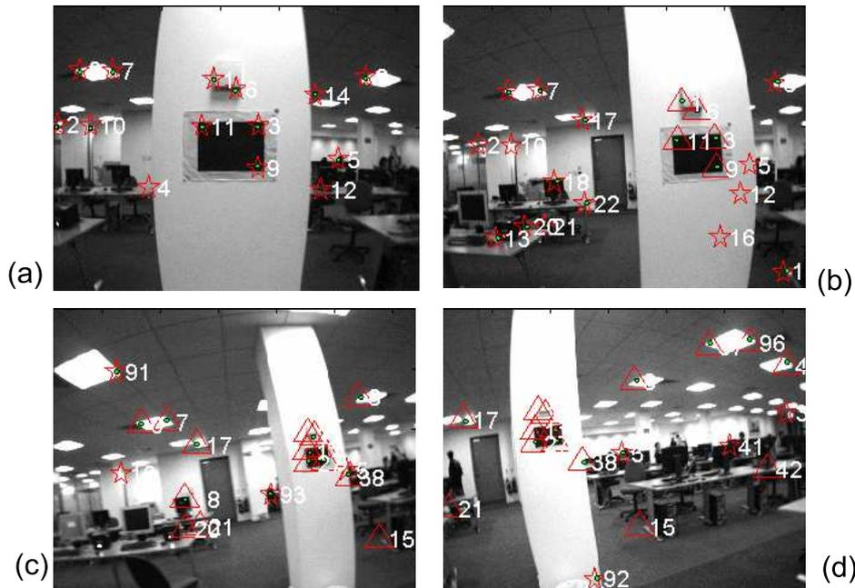
Figure 3.15: Parametrization switching seen in image space: points coded in inverse depth ( $\star$ ) and coded in XYZ ( $\triangle$ ). (a) First frame, with all features in inverse depth. (b) Frame #100; nearby features start switching. (c) Frame # 470, loop closing; most features in XYZ. (d) Last image of the sequence.
