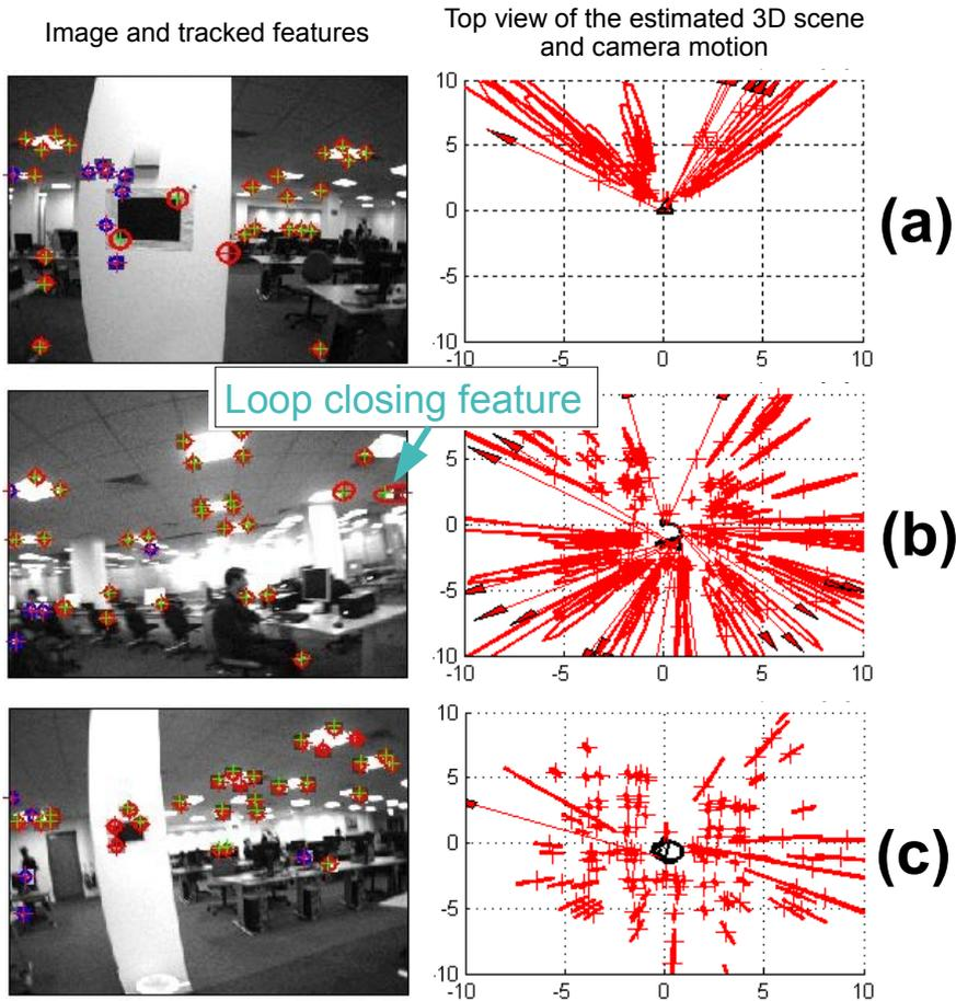
Figure 6.6: (a) Image and 3D estimation at frame 60. (b) Image and 3D estimation at frame 330 of the sequence, when first loop-closure feature (signaled in the image) is detected. (c) Image and 3D estimation at frame 670, the last one of the sequence.
