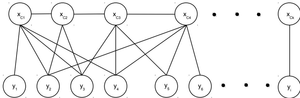
Figure 1.4: Markov random field for sequential SfM or monocular SLAM
