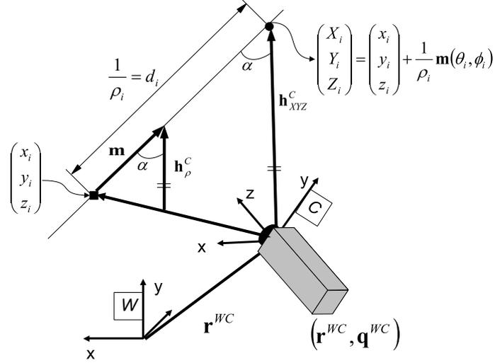
Figure 3.1: Feature parametrization and measurement equation.
