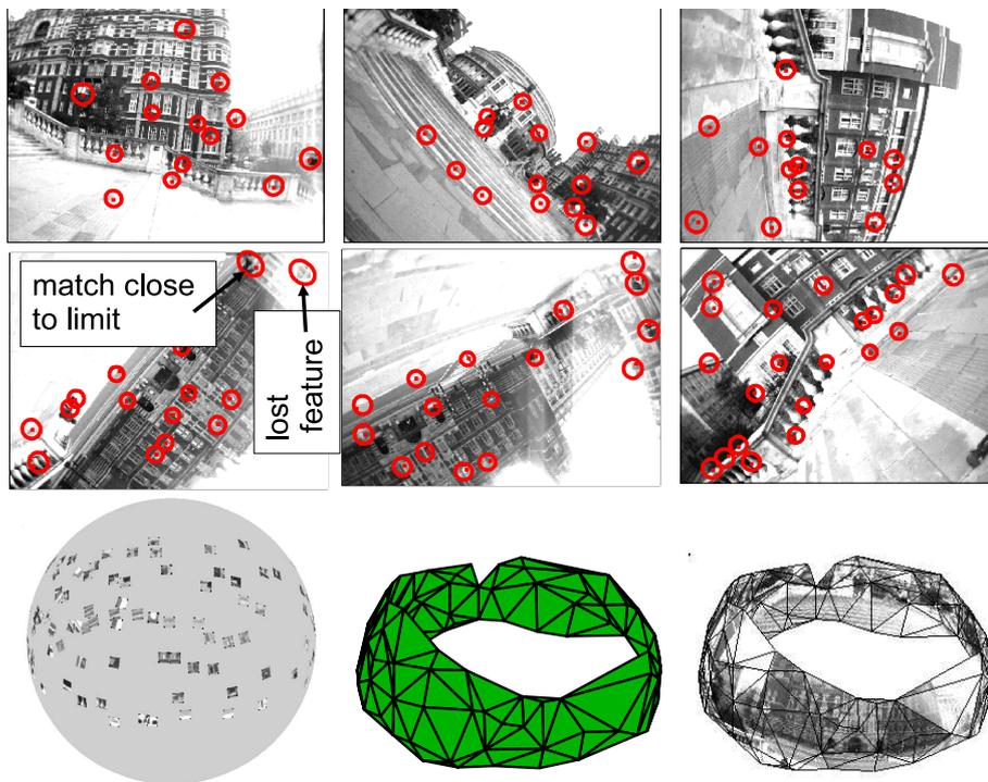
Figure 2.6: 360° pan and cyclotorsion. Top left: first image in sequence. The first image on the second row is at the loop closure point; notice the challenging illumination conditions. Third row: unit sphere with feature patches, triangular mesh and simple texture.
