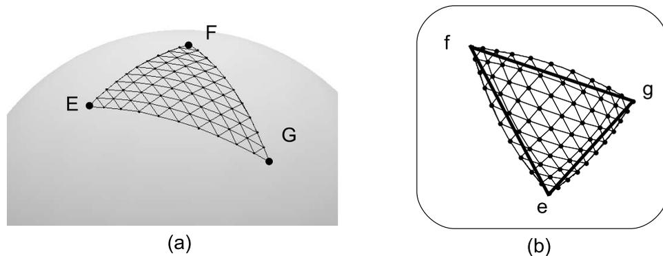
Figure 2.5: (a) Triangular tile defined by map points E,F,G, meshed as subtriangles represented over the unit sphere. (b) Shows the backprojection in the image; notice how the subtriangles also compensate the radial distortion.
