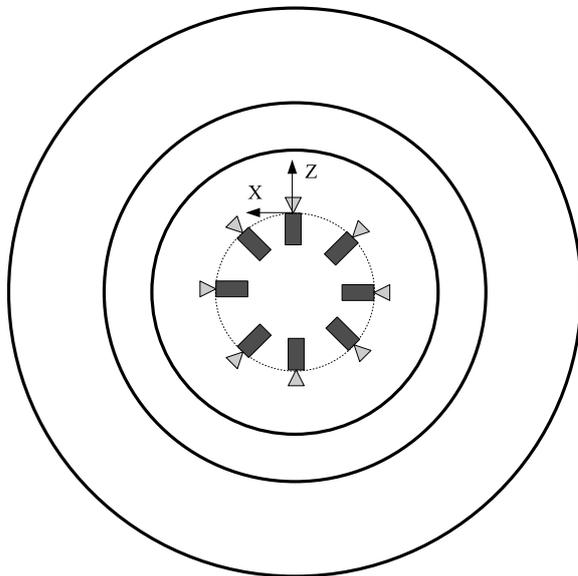
Figure 3.12: Simulation configuration for analysis of parametrization switching in section 3.8.4, sketching the circular camera trajectory and 3D scene, composed of three concentric spheres of radius 4.3m, 10m and 20m. The camera completes two circular laps in the  $(XZ)$  plane with radius 3m, and is orientated radially.
