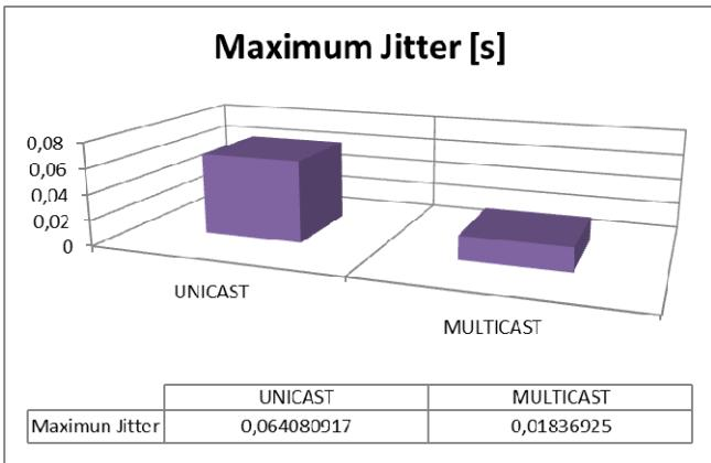
Fig. 4 Maximum jitter in the unicast o multicast traffic
