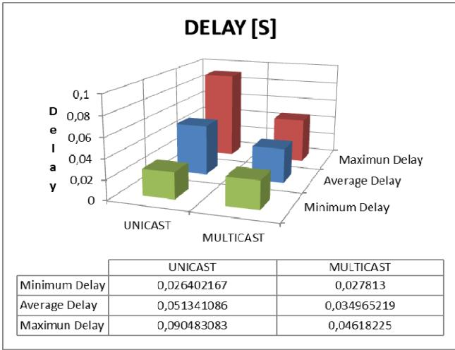
Fig. 3 Average, minimum and maximum delay in the unicast o multicast traffic
