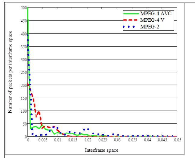
Fig. 7 Distribution of the packets grouped by interframe spaces by coded for unicast traffic in the server
