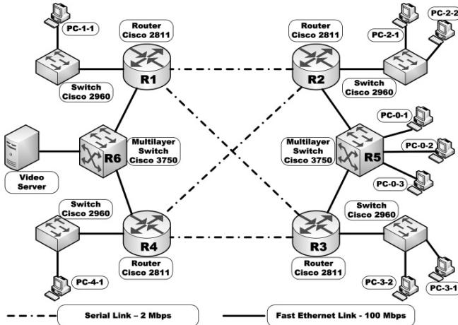
Fig. 1. View of the topology of the WAN test bed.
