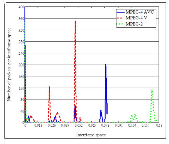
Fig. 6 Distribution of the packets grouped by interframe spaces by codecs for unicast or multicast traffic in PCs
