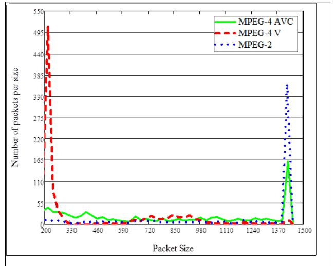
Fig. 5 Distribution of the packets grouped by size for codecs for unicast or multicast traffic in PCs
