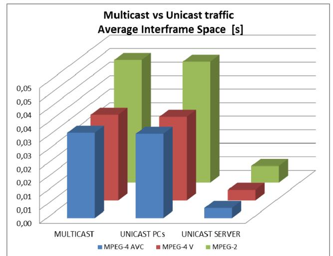
Fig. 2 Average interframe spaces in the unicast o multicast traffic
