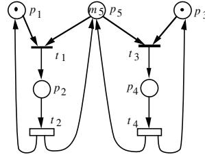
Figure 8.2: A net system whose visit ratios depend on the structure, on the routing at conflicts, on the initial marking, and on the firing times.
