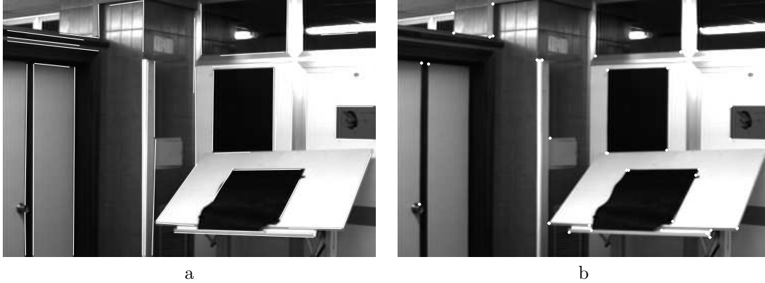
Figure 1: a.- Image of the laboratory with the lines extracted (filtered in gradient and length). b.- Characteristic points selected along the lines.
