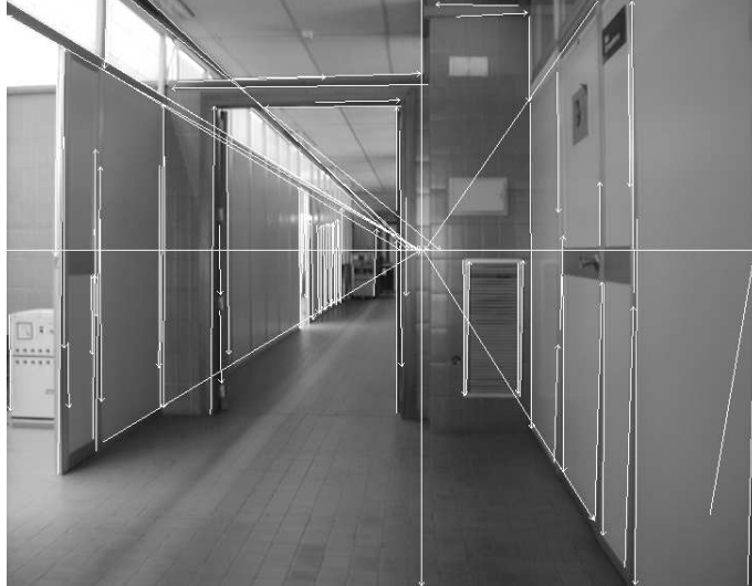
Figure 6: The intersections of significant lines and the line of the horizon provide an estimation of their 3D direction.
