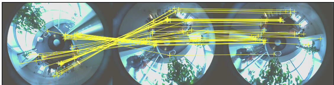
Fig. 6. TEST 2. Corridor (room D) - images D00 D02 D05: 8 robust SURF matches.
