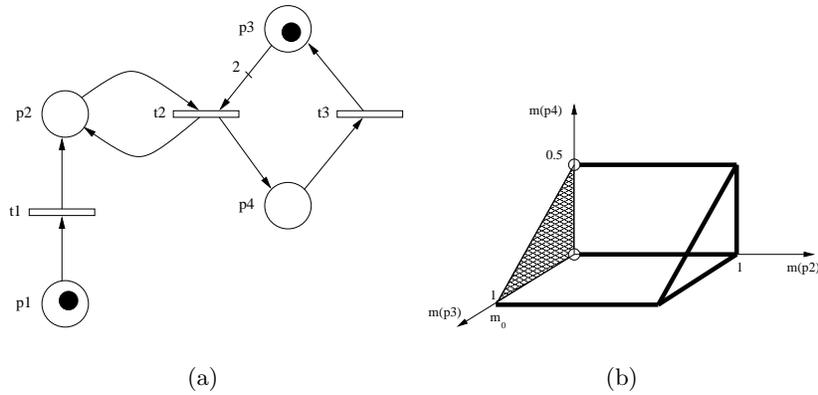
**Fig. 1.** (a) Autonomous continuous system (b) Lim-Reachability space
