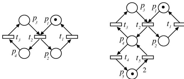
Fig. 4. Two continuous systems for which either not every transition is fireable (left) or the net is not consistent (right), and  $\text{RS}_C(\mathcal{N}, \mathbf{m}_0) \neq \text{LRS}_C(\mathcal{N}, \mathbf{m}_0)$ .
