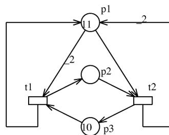
Fig. 14. If  $\lambda[t_1] = 2.25$  and  $\lambda[t_2] = 1$ , the throughput as continuous is not an upper bound of the throughput as discrete.
