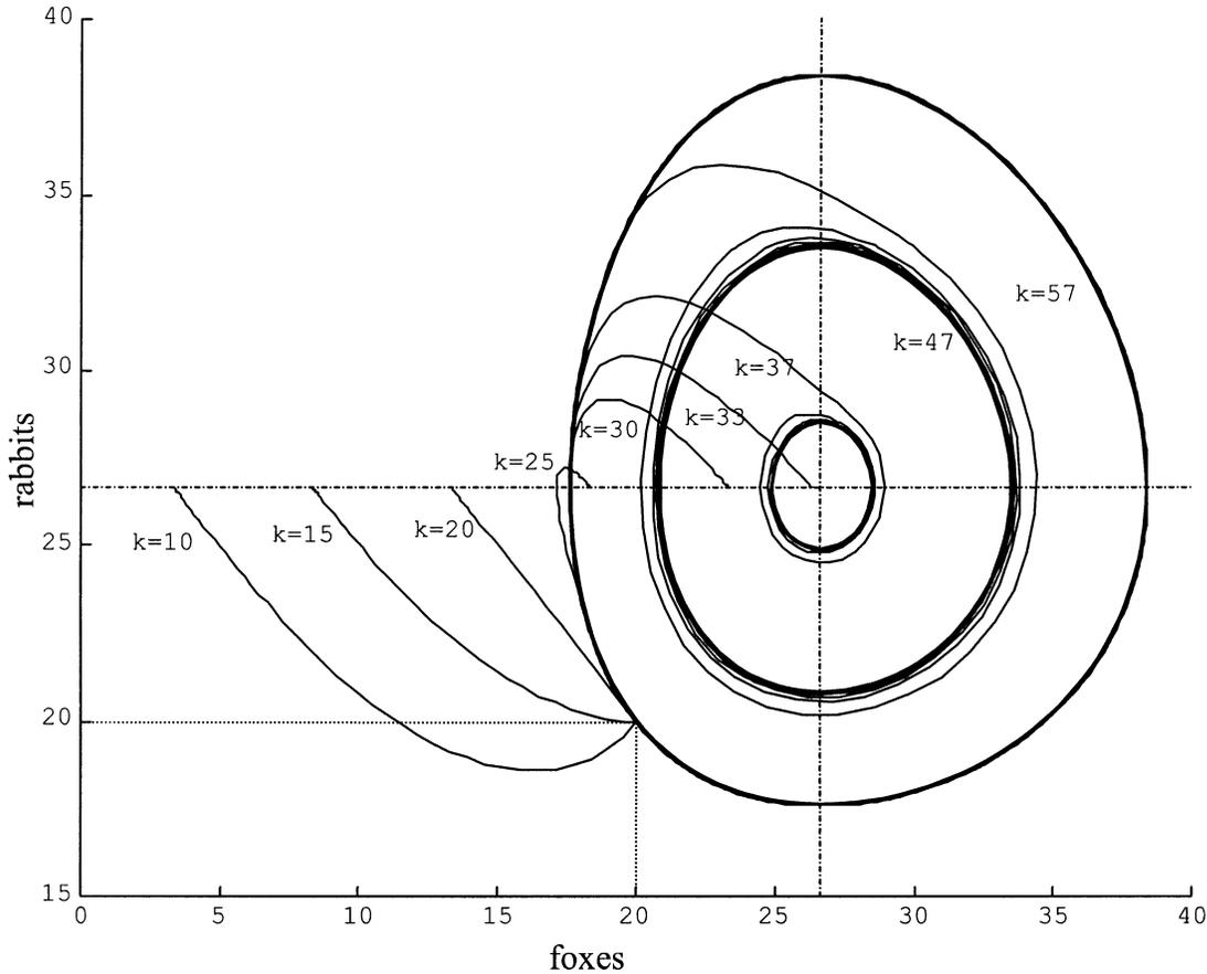
Fig. 12. Trajectories obtained with  $\lambda[t_1] = \lambda[t_2] = 20$ ,  $\lambda[t_3] = 0.75$ ,  $\alpha = 2$ ,  $\mathbf{m}_0[r] = \mathbf{m}_0[f] = 20$ ,  $\mathbf{m}_0[\sim f] = 40$  and  $\mathbf{m}_0[\sim r] = k$ .
