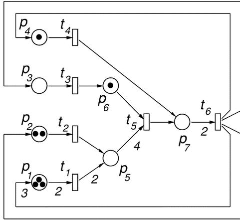
Fig. 7. Choice-free system modeling a manufacturing application [39].
