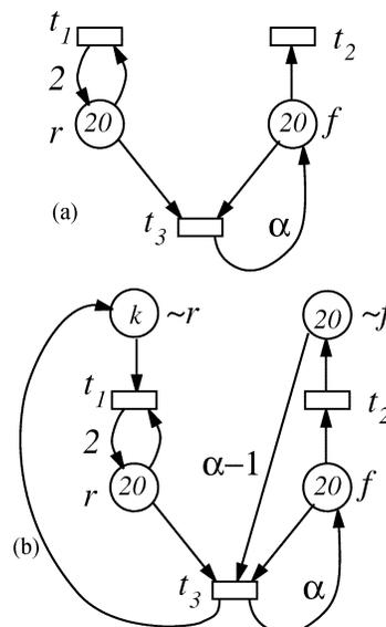
Fig. 11. Place/transition net systems that correspond to the colored PN in Fig. 10, with  $\alpha_r = 0$ ,  $\alpha_f = \alpha$ ,  $\beta_r = 2$ ,  $\beta_f = 0$ , and  $|\Pi| = |\Delta| = 20$ . They can be seen either as discrete or as continuous PNs.
