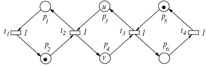
Fig. 8. In this live and bounded marked graph, with  $\lambda = 1$ , the throughput on the steady state depends only on  $k = u + v$ . However, if  $k > 1$  the marking in the steady state is not completely defined by the throughput vector. (Note: if  $k < 1$ , then  $u = v$ ).
