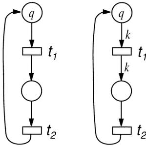
Fig. 1. Two bounded net systems. The one on the right is live as discrete if and only if  $q \geq k$ , but it is live as continuous simply if  $q > 0$ .
