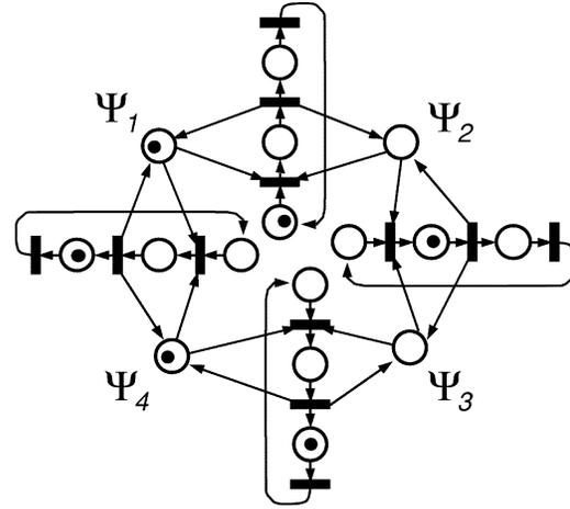
Fig. 9. Place/transition net system of the four philosophers problem. Left and right forks ( $\Psi_i$ ) are taken at the same time.
