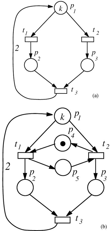
Fig. 6. A structurally nonlive PN (a) and a structurally live PN (b).
