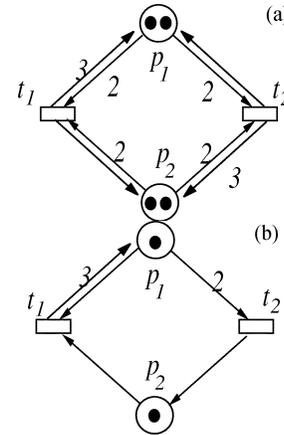
Fig. 2. Two bounded and strongly connected net systems which behave in very different ways if they are considered as discrete or as continuous: (a) is nonlive as discrete, but never gets completely blocked as continuous unless an infinitely long sequence is considered; (b) is live as discrete, but nonlive as continuous.
