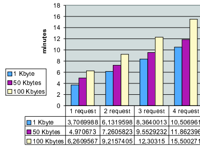
Fig. 19. Response time for an “intelligent Browser”, an “expert user”, a “fast” connection and also different number of request.
