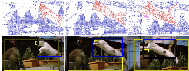
Fig. 3. Localizing objects in videos. (Top) Results of the motion segmentation. (Bottom) Tubes fit to the motion segments (the one selected by our approach is in blue).
