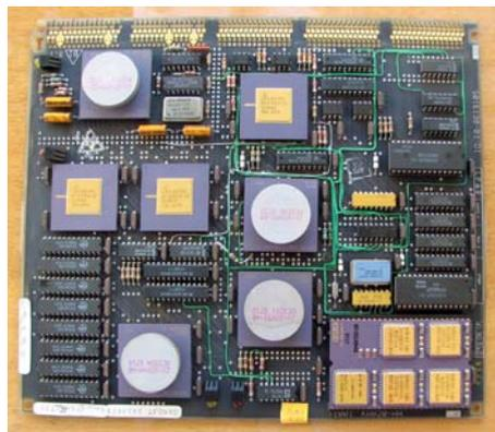
Figura 2.6: Tarjeta KA820-AA. La CPU
