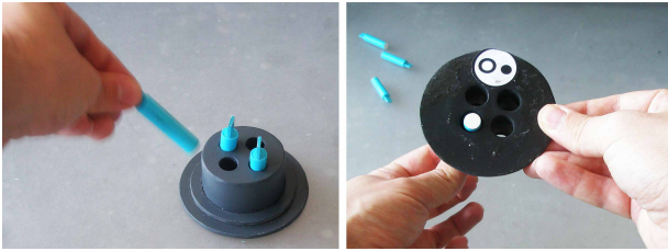
Figure 4. Example of Constraint Token: a “Trivial Pursuit” playing piece (left). Piece’s base with the fiducial and a Simple Token placed inside the constraint (right).
