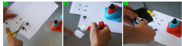
Figure 11. Adapting a playing piece to be used in a tabletop game: Cutting the printed fiducial (a), gluing it (b), attaching the fiducial to the base of the toy (c).
