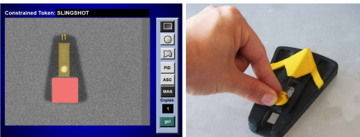
Figure 10. Graphic Assistant: Defining the fiducial area (red square) and the Manipulative Constraint area (yellow rectangle) (left) of a Constraint Token composed of a Simple Token that can be moved along an axis (right).
