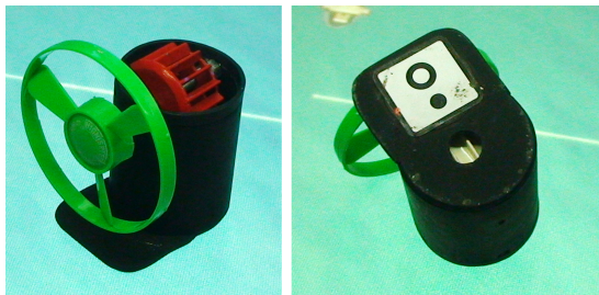
Figure 16. Pirates' Fan toy modeled as Constraint Token (left) with a fiducial and an associative area in its base (right).
