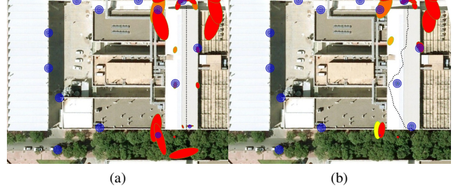
Fig. 2: Comparison between the paths followed by the robot. The hypotheses maintained by the filter are represented as ellipses. The colors indicate the weight of the hypothesis (the redder, the lower). (a) non-active control. (b) active sensing control.
