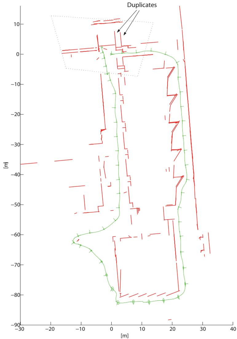
**Figure 3.5:** Classical EKF-SLAM algorithm with an absolute representation. Observe that the vehicle location uncertainty (extremely small ellipses) is incompatible with the real error, especially in the top left part of the figure, where clearly, multiple hypotheses for the same feature appear.
