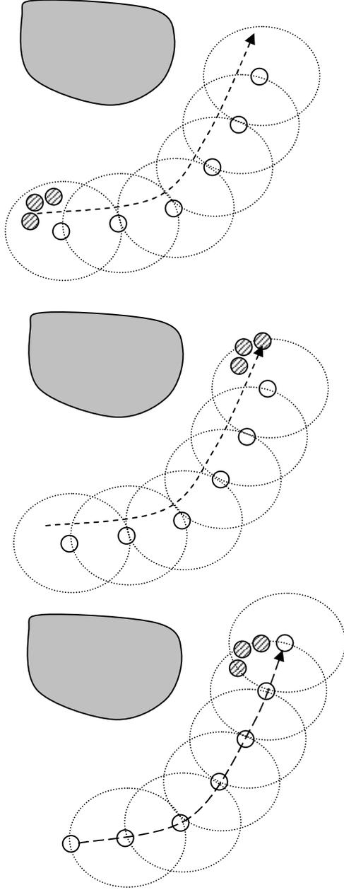
Fig. 2. Trail of active robots. First, the active robots (white circles) are deployed along the path. Then the passive robots (dashed circles) travel along the path with the tracking of the active robots. If the number of active robots is not enough to cover all the distance, the process is repeated from the first point since the goal is reached. The dotted circles show the range of sensors.
