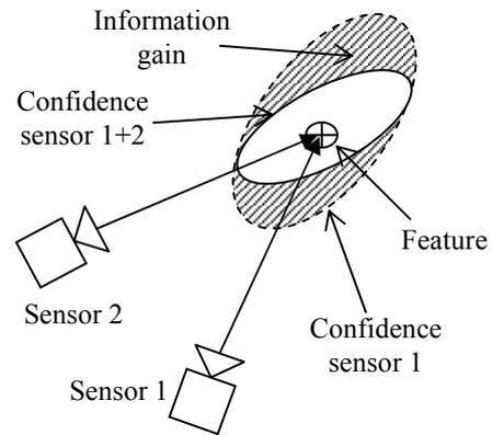
Fig. 1. Dependence between two observations. First, Sensor 1 observes the feature within a confidence interval (dashed ellipse). Finally, Sensor 2 observes the same feature with a confidence interval inside the last one (solid ellipse). The marked area shows the information gain.
