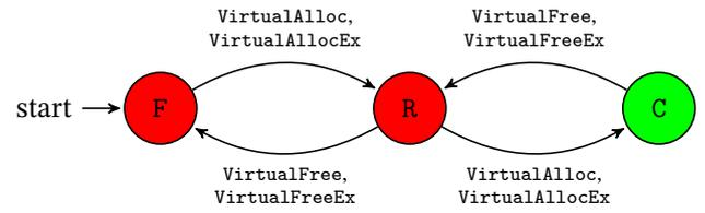
Figure 2: State machine of memory page states in Windows: F (free), R (reserved), C (committed). The state color indicates whether the page is accessible to the process (green) or not (red). Edge labels indicate the Windows system call used to transition between states.
