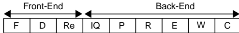
Figure 1 Processor Pipeline. F: Fetch, D: Decode, Re: Rename, IQ: Issue Queue, P: Read Payload, R: Read Register File, E: Execution, WR: Write Register File, C: Commit.
