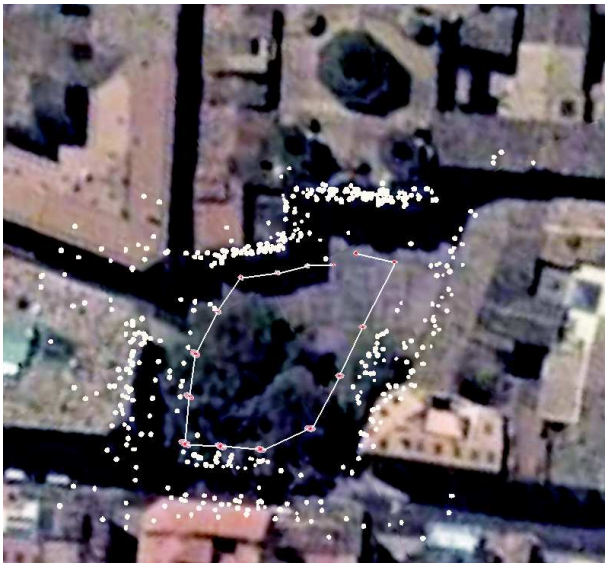
Fig. 11. Final map and trajectory estimates superimposed to an aerial image of the real environment.
