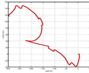
**Fig. 3.** Accumulation of position error relying only on dead-reckoning for a long distance traverse of the B21 mobile robot. The actual vehicle path went down approximately 40 meters, to the left approximately 225 meters, and then back to the origin.
