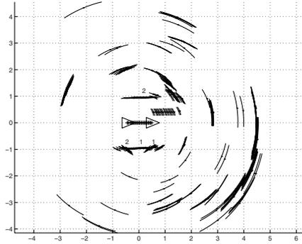
**Fig. 10.** Example of Hough processing to extract point and line features. Sonar returns are processed in a group of twenty-two positions. A voting scheme is performed to find clusters of measurements that hypothesize the existence of point and plane features. For this example, two planes and two points have been found.
