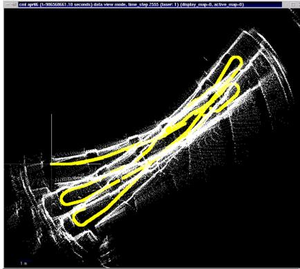
**Fig. 1.** Laser data for a short corridor experiment, referenced to the dead-reckoning position estimate
