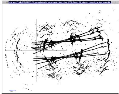
**Fig. 14.** Raw sonar data for corridor experiment, referenced to odometry.
