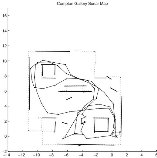
**Fig. 12.** Complete map for the MIT Compton Gallery built from sonar using Hough grouping, Map Joining, and Joint Compatibility.
