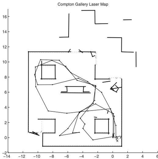
**Fig. 13.** Complete map for the MIT Compton Gallery built from laser data using Robust Statistics, Map Joining, and Joint Compatibility.
