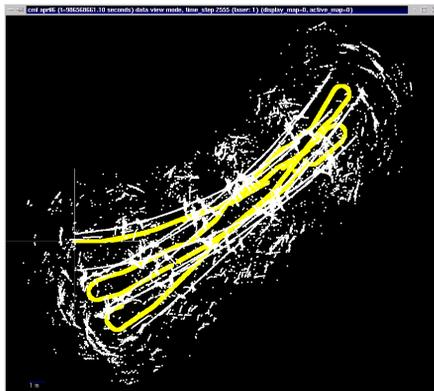
**Fig. 2.** Sonar data for a short corridor experiment, referenced to the dead-reckoning position estimate
