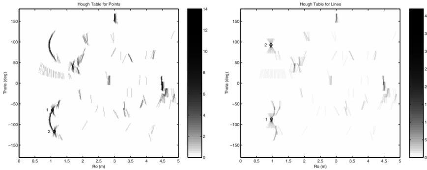
**Fig. 11.** Hough voting table for point (left) and line (right) features.
