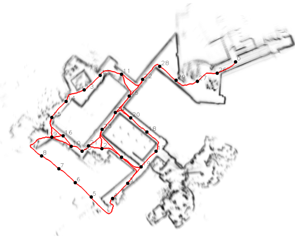
Figure 12. The probabilistic graph for path planning obtained out of the pose graph of the MIT CSAIL dataset with 31 nodes and 40 edges.
