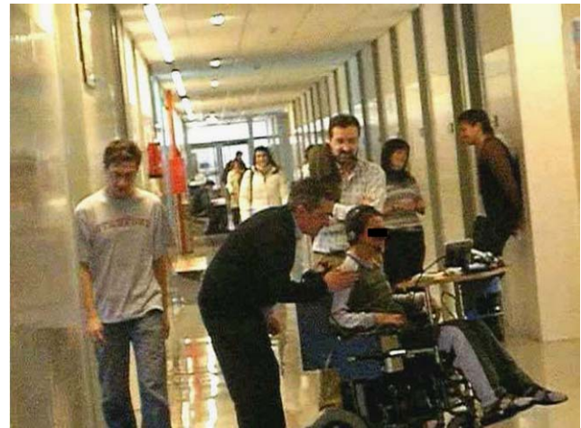
Fig. 2 A child using an autonomous robotic wheelchair in a crowded and populated scenario. The number and dynamics of the moving obstacles is unpredictable. To deal with the motion aspect in these scenarios is the context of this work
