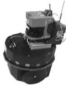
(f) Scout platform (Technical University of Lisbon) Circular differential drive, Ultrasounds
