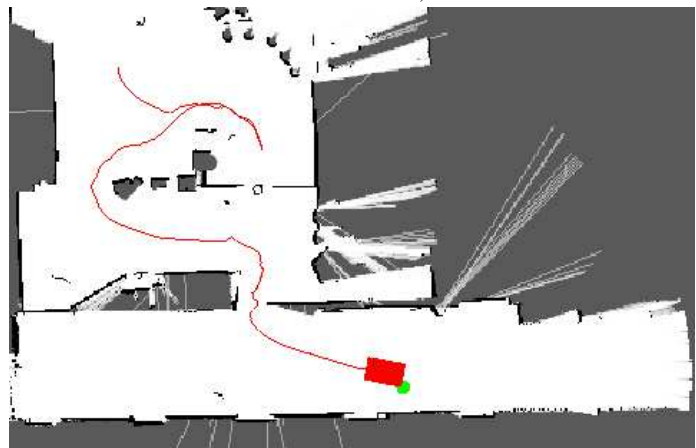
(g) Robotic wheelchair platform (University of Zaragoza) Rectangular differential drive, SICK Laser
