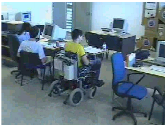
(g) Robotic wheelchair platform (University of Zaragoza) Rectangular differential drive, SICK Laser
