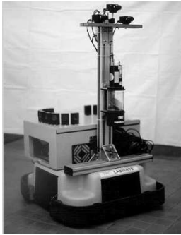
(a) Labmate platform (University of Zaragoza) Rectangular differential drive, TRC 3D laser
