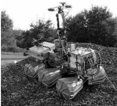
(e) Lama platform (LAAS-CNRS) Rectangular differential drive, stereo vision
