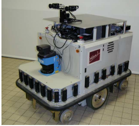
(c) Hilare platform (LAAS-CNRS) Rectangular differential drive, SICK Laser
