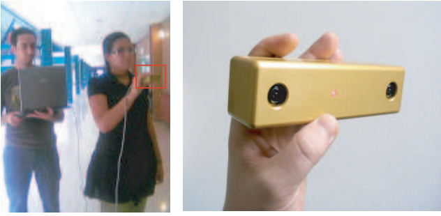
Fig. 1. Bumblebee Stereo vision system used to acquire images sequences. Picture on the left shows the experimental setup during the data acquisition for the indoor experiment.
