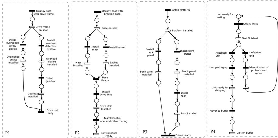
Fig. 3. Main procedures involved in the assembly of a TPL, represented by Petri net structures. P1 is carried out in parallel to the rest, which are carried out in a sequential manner  $P2 \Rightarrow P3 \Rightarrow P4$ .
