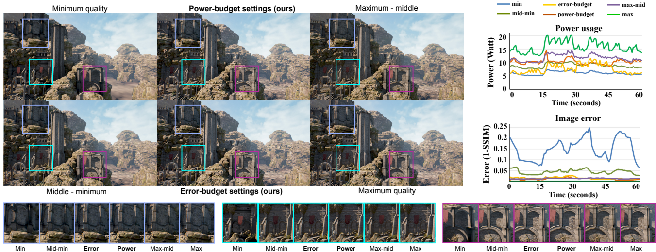
Figure 11: Elven Ruins real-time demo using the Unreal Engine on a desktop PC. We compare minimum, middle-minimum, maximum-middle and maximum quality settings against two modes of our power-optimal rendering framework: Selecting a power budget of 10W, and an error budget of 0.02. Plots on the right show power usage and error during a 60-second camera path. Our framework provides power-error optimized settings under the two different budget modes, while guaranteeing in both cases a visual quality very similar to the maximum settings, and power usage close to the minimum settings. Moreover, our optimized settings outperform manual settings. Please refer to the supplementary video for the full demo.
