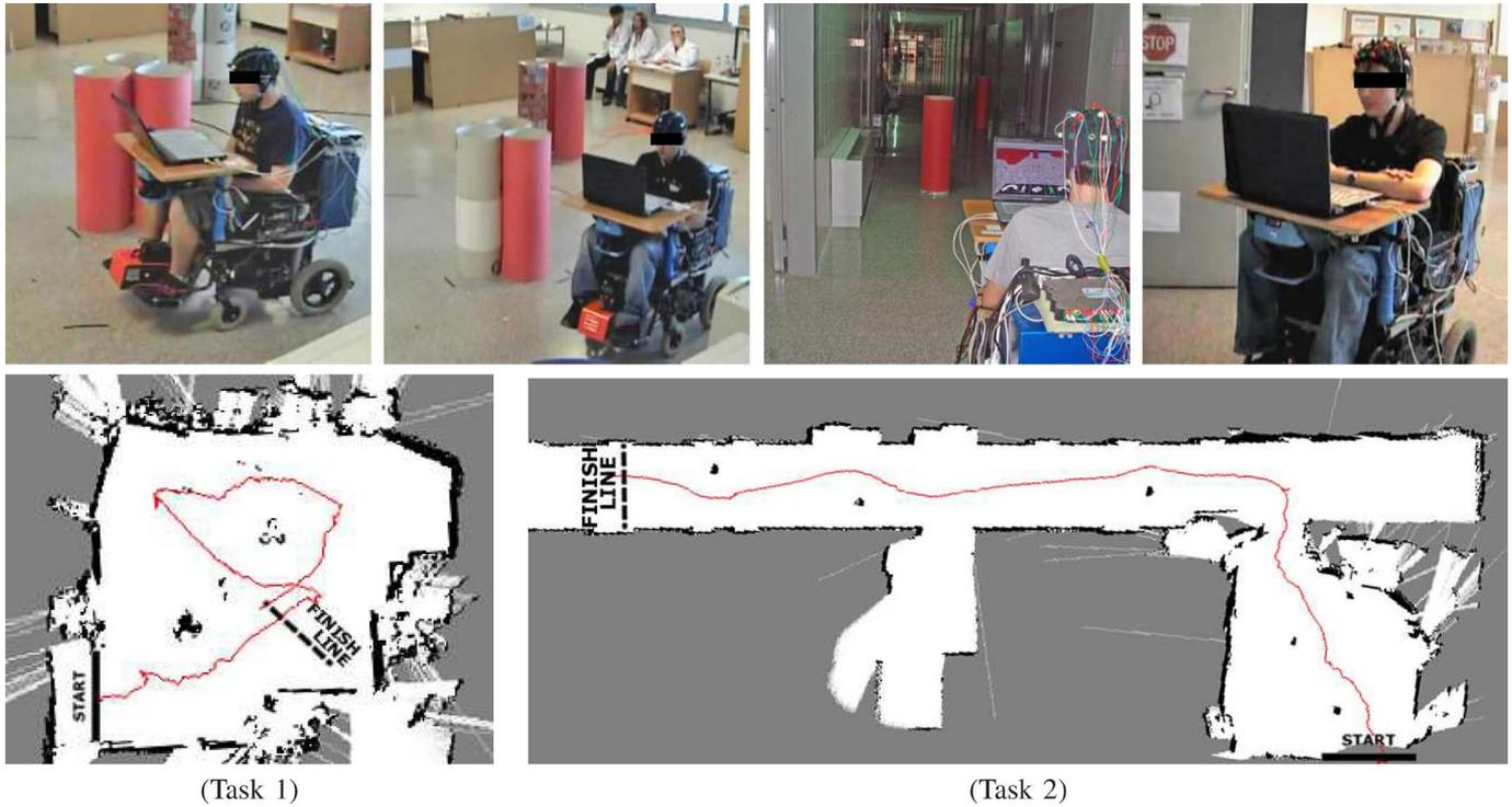
Fig. 7. First row shows snapshots of the experiments with the wheelchair. The first two figures correspond with task 1, and the following two figures with task 2. The second row shows the map generated by the autonomous navigation system and the trajectory of the wheelchair in one real experiment of each task. Black zones indicate obstacles, white zones indicate known areas, and gray zones indicate unknown areas.
