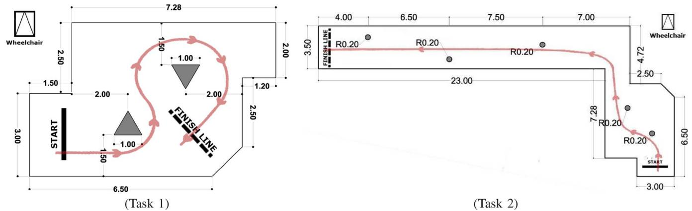
Fig. 6. Objective of task 1 was to leave the start area and to reach the finish line by passing the first triangle on the left-hand side, passing between the two triangles, and passing the last triangle on the right-hand side. The objective of task 2 was to simply reach the finish line. An example of a possible path is marked. All measures are in meters and the wheelchair is to scale. The shaded objects represent static obstacles.
