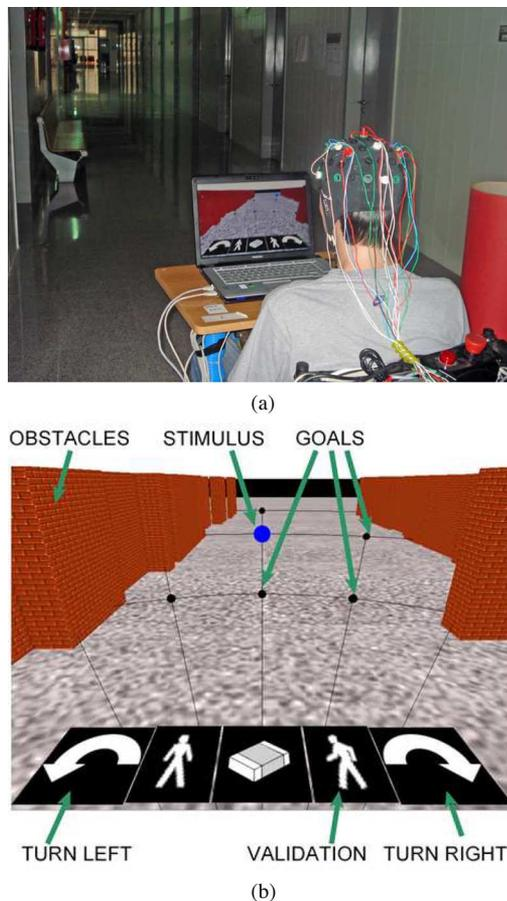
Fig. 3. (a) Snapshot of a participant navigating along a corridor. (b) Information represented in the visual display, which is an environment abstraction displayed from the user's point of view.
