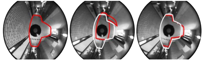
Figure 9: Left: Hypothesis of image I (red). Center and right represent two homography cases where the white contour represents hypothesis of image I' and red contour is the hypothesis projection from I to I' . Center: Case where homography does not perform well. Right: Case of the best homography.
