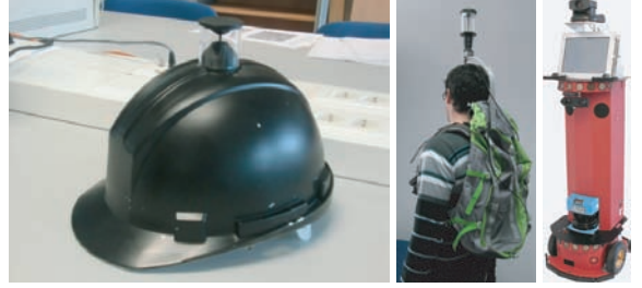
Figure 11: Devices used for omnidirectional image acquisition: a helmet (left), a backpack (center), and a mobile robot (right).
