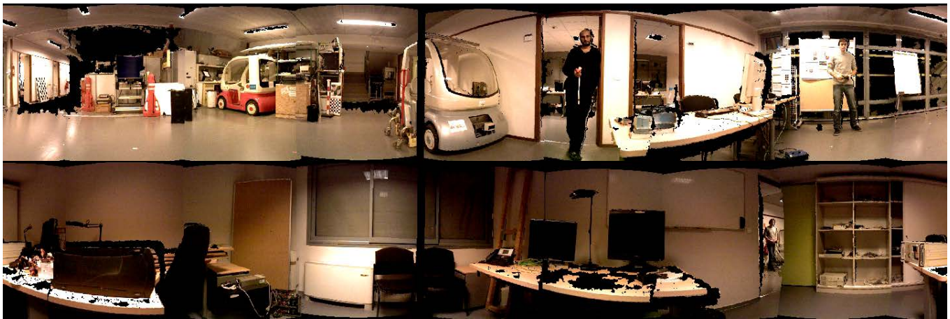
Fig. 7: Panoramic views from two different scenes obtained with the 8 RGB-D camera rig. The views have been obtained by reprojecting the 3D points transformed to a common reference frame with the relative poses obtained following our multi-camera calibration method.
