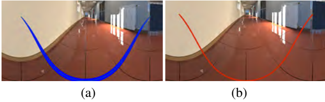
Fig. 4. Region around a line projection defined by a given distance. (a) Metric distance \mathbb{E}^3 from ray to line. (b) Proposed metric distance on the image.
