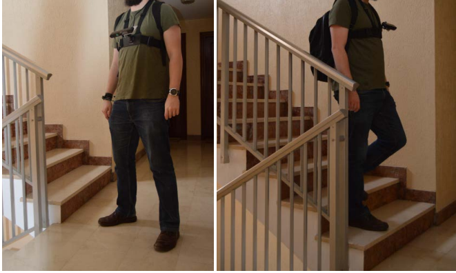
Fig. 1. Photos of the current wearable camera system while detection (left) and traversal (right). The camera is placed on the chest, pointing downwards. The computations are performed in a laptop carried in a backpack.
