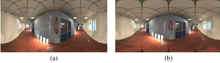
Figure 5.2: (a) Circular panoramic image with R_c = 0.5m (Non-central). (b) Circular panoramic image with R_c = 0m (A central spherical panoramic image).
