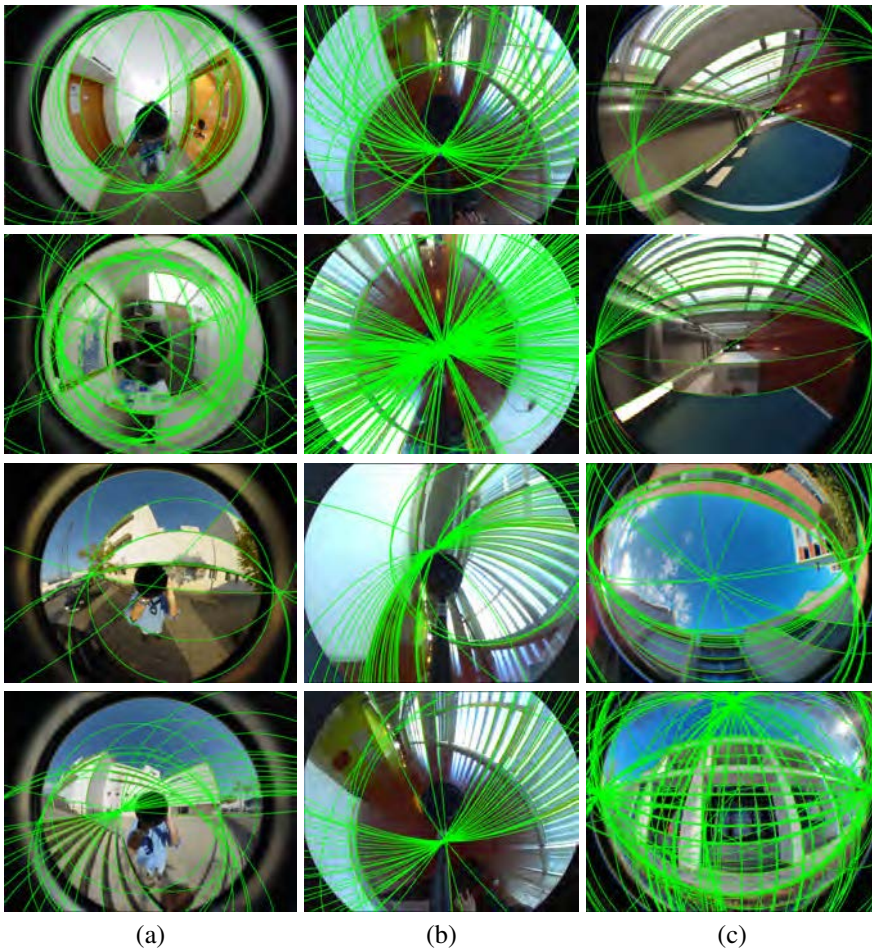
Figure 3.20: Line extraction on uncalibrated omni-images (3-points algorithm). (a) Paracatadioptric. (b) Hypercatadioptric. (c) Equiangular-Fisheye
