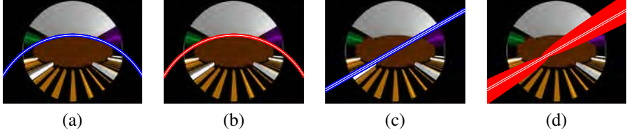
Figure 2.3: Region defined by a metric threshold of 20 pixels surrounding a conic. (a) Ellipse case using metric distance. (b) Ellipse case using Sampson distance. (c) Hyperbola case using metric distance. (d) Hyperbola case using Sampson distance.
