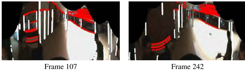
Figure 2.16: Panoramic representation of several full-rectified frames. Vertical lines are shown in white and horizontal ones in red. The horizontal vanishing point is aligned to the image center.
