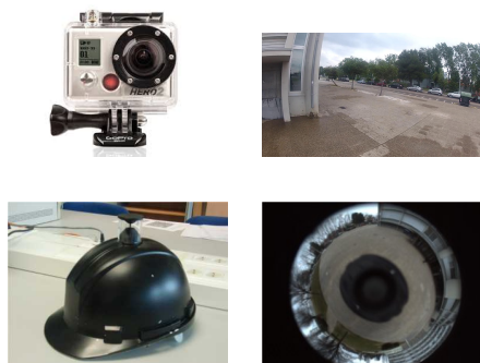
Figure 1. Devices used in our experiments. On top, GoPro Hero 2 wide angle camera. On bottom, our helmet with catadioptric camera consisting on a conic mirror and a VS-C14U-80-ST catadioptric camera.
