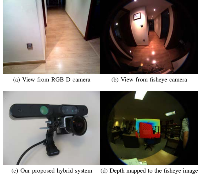
Fig. 1: (a) Scene view from a conventional RGB-D camera. (b) Same scene view from a fisheye camera. (c) Our proposal: hybrid camera system with Depth and Fisheye. (d) After the calibration we can map the depth to the whole scene image.
