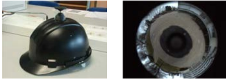
Figure 7: Our helmet with catadioptric camera and example of images taking during the sequence.
