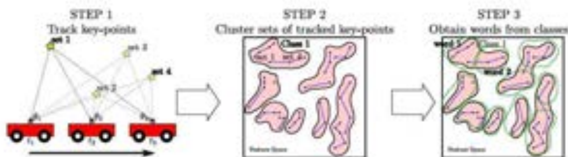
Figure 5.1: Diagram of our novel vocabulary construction method. During the acquisition, extracted image key-points are tracked. All the image appearances and azimuth angle values of these key-points are stored and grouped together under the same set number. These sets of tracked key-points are later clustered into classes, with the elements in each class representing the same environment element. Finally, words are extracted running a clustering for each of the obtained classes.
