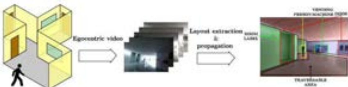
Figure 6.1: Our goal is to process video acquired from a wearable camera to obtain the 3D layout of the scene in each frame (Red: floor and ceiling; Green and Blue: walls from different orientations). This layout information is a strong prior to facilitate the detection of other scene details: persons, signs, doors or the traversable area.
