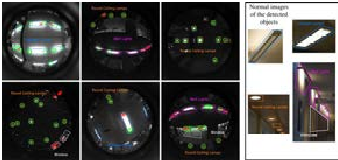
Figure 5.13: Examples of objects found in the dataset. Green circles mark correct assignments and red crosses show incorrect ones. The colored shapes show the labeled areas: Round Ceiling Lamps (orange); Halogen Lamps (blue); Wall Lights (magenta); Windows (white). Matching threshold is set to 0.15. For clarity, some conventional images of the objects in the environment are shown on the right of the figure. (Best seen in color).
