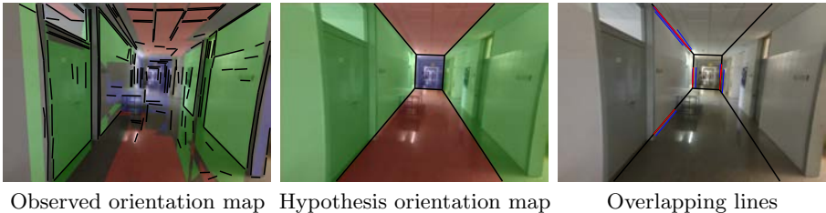
Fig. 4. Evaluation of the hypotheses. The observed orientation map, computed from the detected lines, and the hypothesis orientation map are compared to compute S_{omap} . S_{overlap} is computed as the length of overlapping (red) divided by the total length of the hypothesis lines (black). Blue lines are the detected lines that are parallel and close to the model lines. (Best seen in color).
