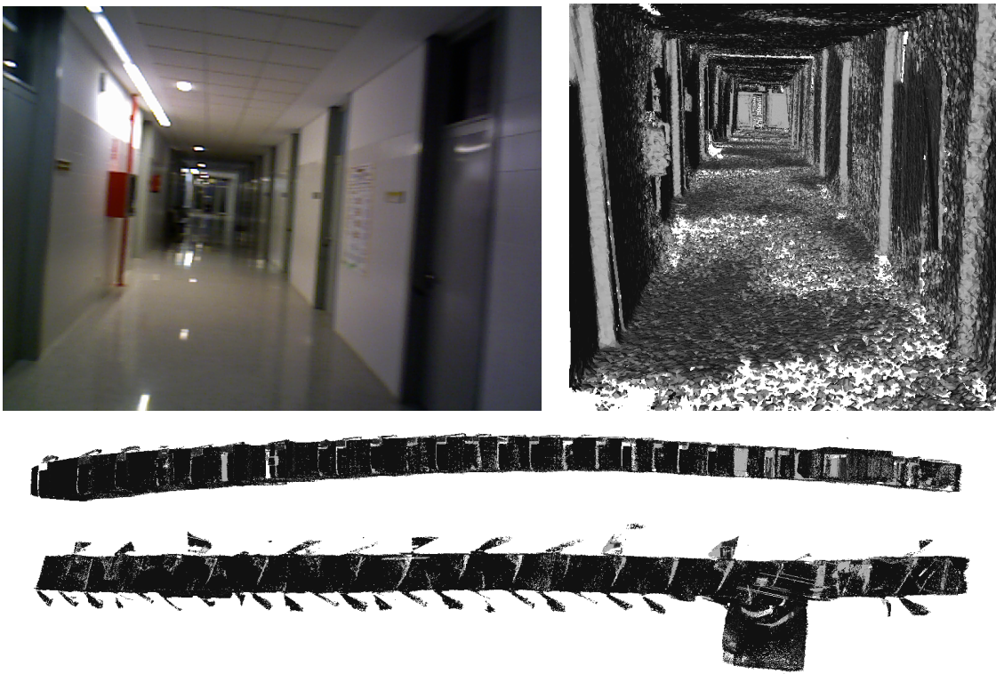
Figure 4.12: (Top-left) RGB image of the corridor, (Top-right) KinectFusion 3D reconstruction with our visual odometry method, (middle) side view and (bottom) plant view of the complete 3D mesh. Note the challenging of the sequence due to the poor texture of the corridor and light reflexes.
