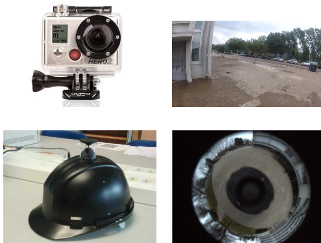
Figure 3.1: Devices used in our experiments. On top, GoPro Hero 2 wide angle camera. On bottom, our helmet with catadioptric camera consisting on a mirror and a VS-C14U-80-ST catadioptric camera.
