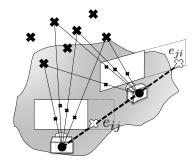
Fig. 1: The robots use the epipoles between their images to compute the control input.
