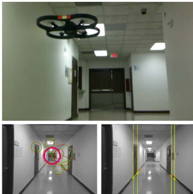
Fig. 1: Our method uses vistas (bottom left) to maintain long-term orientation consistency and relies on a map of Wall-Floor Intersection Features (bottom right) to infer the scene structure. We present our results in an indoor setting using a Parrot AR.Drone (top).
