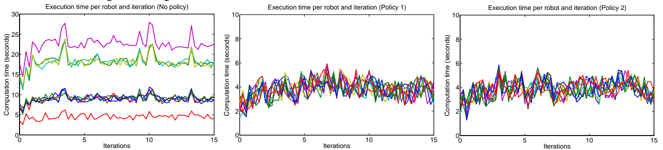
Fig. 6: Computational time spent by each robot at each iteration: without any policy to select the neighbors (left), with the policy to choose the neighbor that was not selected for the longest time (middle) and with the policy to choose the neighbor with the most misalignment (right). As we can see, when the robots use a policy, all of them spend approximately the same computational time, whereas without a policy each robot requires a different time depending on its neighbors.
