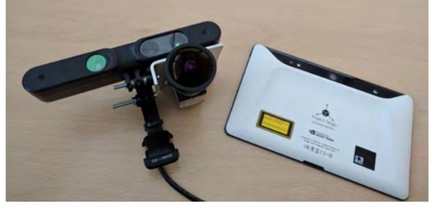
**Figure 13:** The two devices used to collect the data for our experiments. On the left, an RGB-D camera (ASUS Xtion Pro Live) with an adjacent fisheye camera. On the right, the Google Tango Development Kit.
