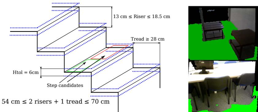
**Fig. 3:** Representation of the measurements of a step according to the Technical Edification Code from Spain (left). In green, the portion of the ground which can be walked over as it has no obstacles above (right).
