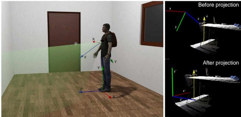
**Fig. 1:** Wearable camera location and axis position before ( $XYZ$ ) and after ( $X'Y'Z'$ ) the projection to the ground in a 3D render (left). Point clouds from a real case scenario, where the white points on the floor are those which form the best floor candidate plane and the yellow arrow is the corresponding normal (right).
