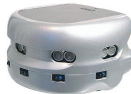
Fig. 9. Khepera III robot from K-Team S.A.
