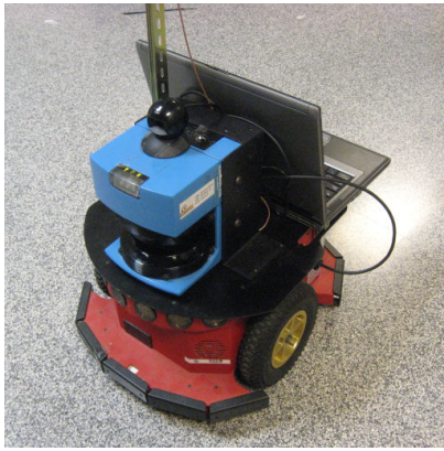
Fig. 11. The experimental platform with a camera and laptop onboard.
