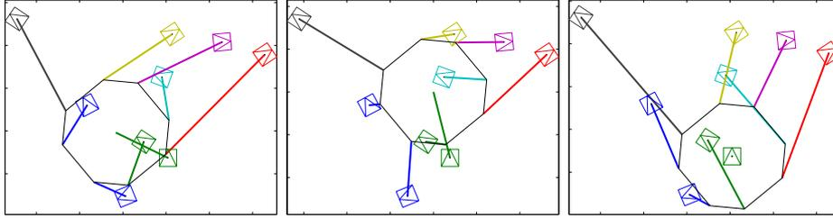
**Fig. 1.** Comparison of the desired image location for the robots provided by the goal homography in different cases for some instant time. The control law is performed without considering the centroid of the robot distribution (left), whereas it is considered in the next case (center). The last case translates the centroid of the desired robot locations to the leader (right).
