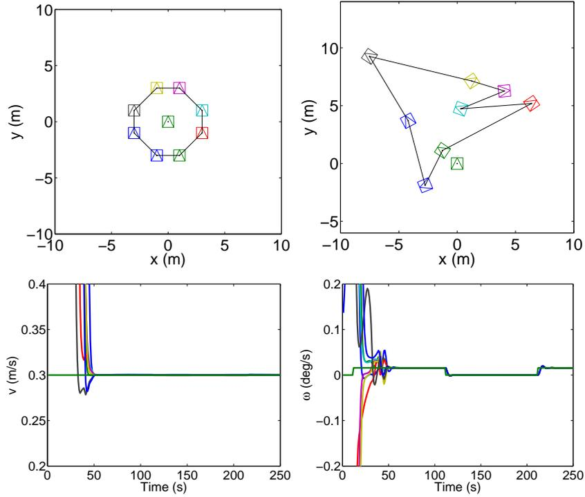
**Fig. 3.** The desired configuration of the robots and their initial positions for the simulation presented are depicted, respectively, in the first row. The robots are distributed in the desired formation forming an octagonal shape with the leader robot in the centre. The linear and angular velocities given by the controller to follow the leader in formation are depicted in the second row.
