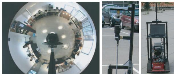
Fig. 10. Example image (left), omnidirectional camera (center) and complete setup (right) used for the experiments.
