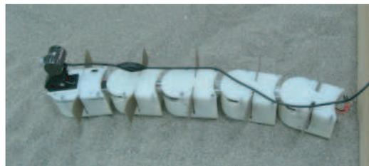
Fig. 1. The Nereisbot undulatory robotic prototype, with an on-board camera mounted on its head link.
