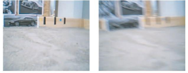
Fig. 6. Two images acquired with the on-board camera and demonstrating the blurring effect caused by the fast head yaw during undulatory movements of the robot. The image on the left has been acquired at the limit of the head yaw, when the lateral velocity is instantaneously zero, and is therefore significantly sharper.
