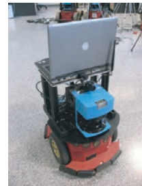
Fig. 11. The experimental platform, a Pioneer P3-DX from ActivMedia.
