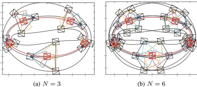
Fig. 7. *The image shows a simulation that includes and tracks a target with ellipsoidal motion. Two cases are shown from left to right: the number of robots chosen is  $N = 3$  and  $N = 6$ , respectively. The simulation depicts the movement of the target and the robots surrounding it. In addition, the polygon of the formation and the wedges (FOV) of each robot are also represented during some instants of time.*
