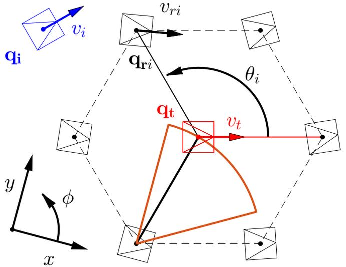
Fig. 3. Constant scale formation strategy: The parameters involved the multi-robot strategy are depicted. We need to define the reference trajectories:  $q_{r_i}$  for the robots  $q_i$  to maintain a circular formation enclosing the target  $q_t$  and maintaining FOV constraints. Each robot  $q_i$  will track its reference trajectory  $q_{r_i}$ . The FOV of the onboard fixed camera of one robot is also shown.
