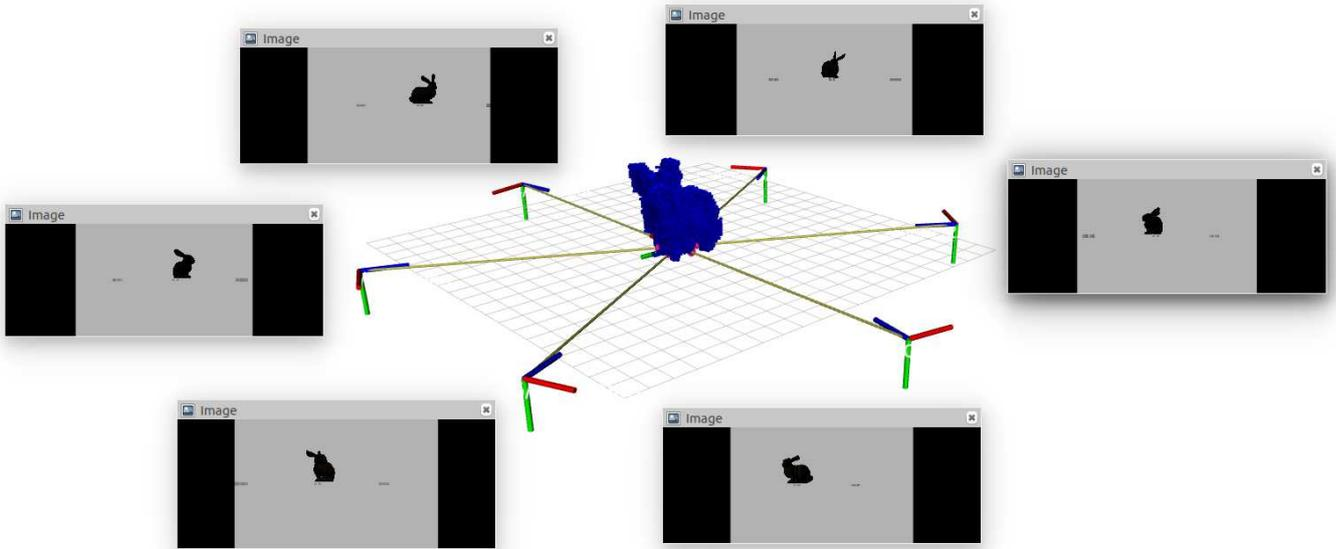
Fig. 6. *Reconstruction in simulation: The full model for the Stanford bunny dataset is observed, where the occupied voxels are painted in blue. The multi-camera hexagonal-shape formation is also visualized. In the task of instantaneous perception of an object, the field of view of each camera covers a portion of the surface of the object at each instant of time. By merging these observations, the object is fully perceived.*
