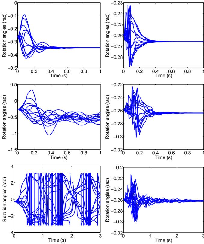
Fig. 6. Estimation of the rotation angle by each agent under time delays: left column, no delay compensation; right column, delay compensation with delay mismatch of 15ms. Top:  $\bar{\tau} = 100ms$ , Middle:  $\bar{\tau} = 200ms$ , Bottom:  $\bar{\tau} = 500ms$ .
