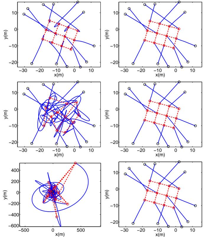
Fig. 5. Paths followed by each agent under time delays: left column, no delay compensation; right column, delay compensation with delay mismatch of 15ms. Top:  $\bar{\tau} = 100ms$ , Middle:  $\bar{\tau} = 200ms$ , Bottom:  $\bar{\tau} = 500ms$ .
