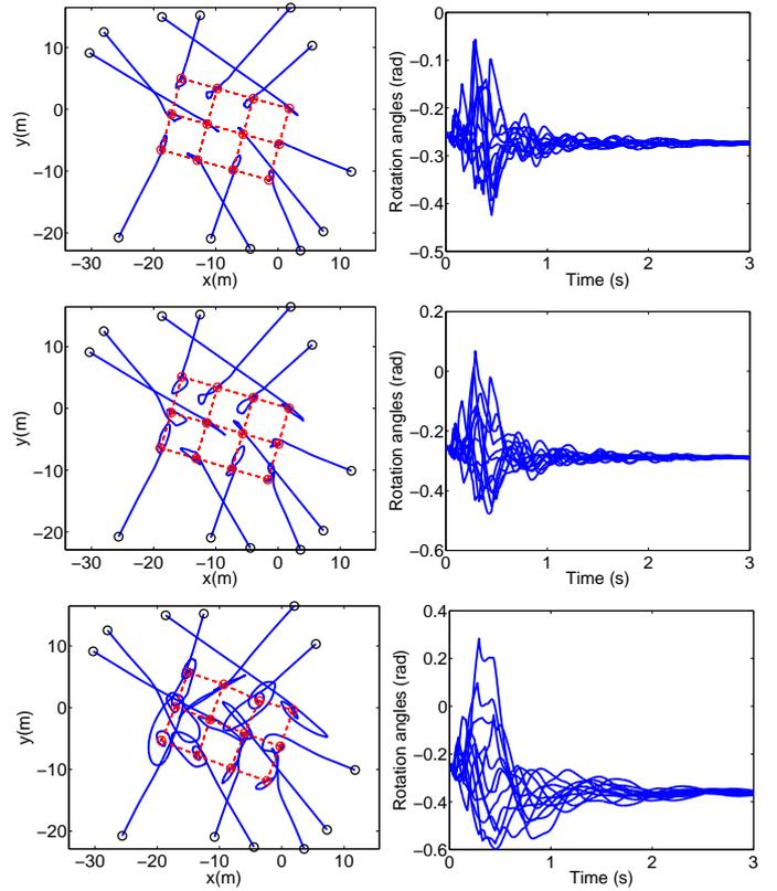
Fig. 9. Simulation results with upper bound delay  $\bar{\tau} = 500ms$  and bigger delay mismatches: left column, trajectories followed by each agent converging to the desired geometric configuration; right column, estimation of the rotation angle by each agent. Top:  $e_\tau = 75ms$ , Middle:  $e_\tau = 125ms$ , Bottom:  $e_\tau = 250ms$ .
