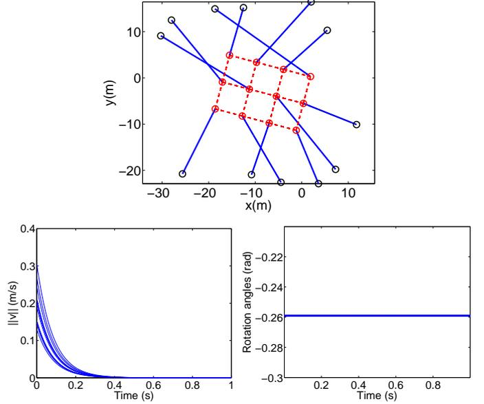
Fig. 4. Simulation results using the proposed control scheme with time delays  $\tau_{ki} = \bar{\tau} = 500ms$  and no delay mismatches ( $\hat{\tau}_{ki} = \tau_{ki}$ ). Upper figure: trajectories followed by each agent converging to the desired geometric configuration. Lower left-side: Norm velocities of each agent, Lower right-side: Estimation of the rotation angle  $\hat{\alpha}_i = \hat{\alpha}_0 = -0.2591$ , computed by each agent.
