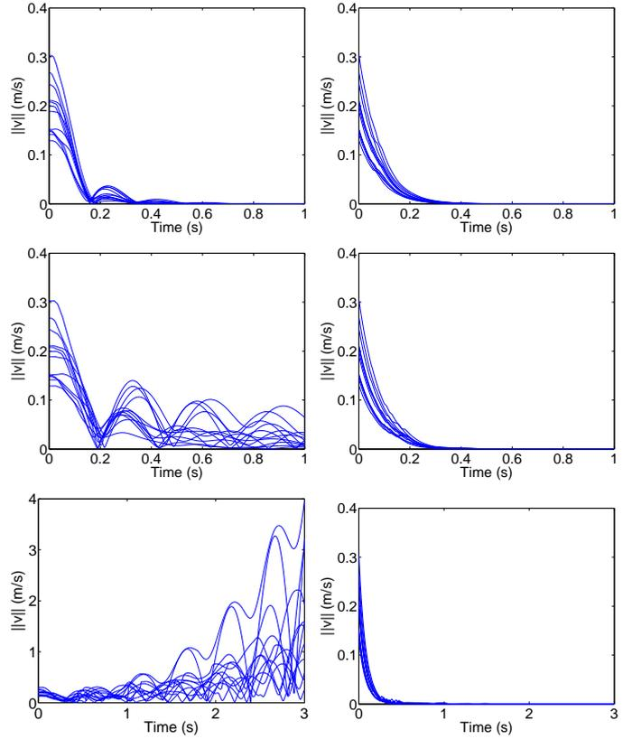
Fig. 7. Norm velocities corresponding to each agent under time delays: left column, no delay compensation; right column, delay compensation with delay mismatch of 15ms. Top:  $\bar{\tau} = 100ms$ , Middle:  $\bar{\tau} = 200ms$ , Bottom:  $\bar{\tau} = 500ms$ .
