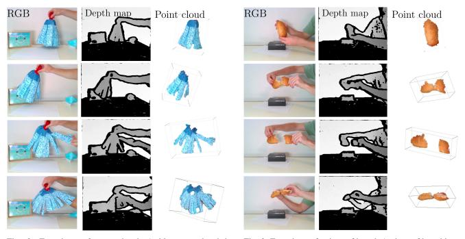
Fig. 2: Experiment 2: mop head. A blue mop head is manipulated avoiding confusion with the background.
