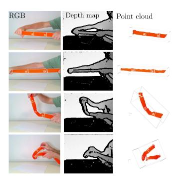
Fig. 1: Experiment 1: elastic band. An orange elastic band is stretched and bent.
