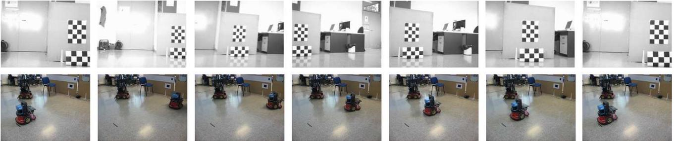
Fig. 10. Sequence of some images taken from the robot camera (1st row) and from an external camera (2nd row) during the real experiment. The first is the target image, the second is the initial and the last is the image at the end of the motion. The robot behind is not involved in the experiment.
