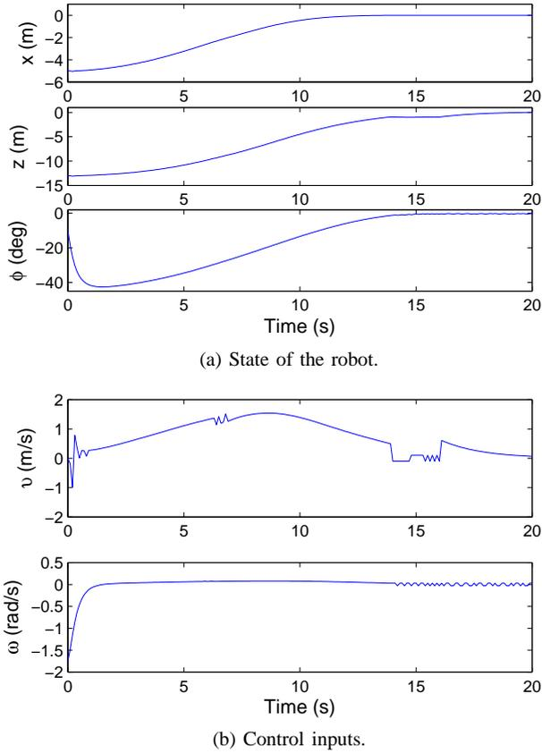
Fig. 6. Simulation results: evolution of the state of the robot and velocities for the case 3 in Fig. 5, where the singularity is crossed in the first seconds.
