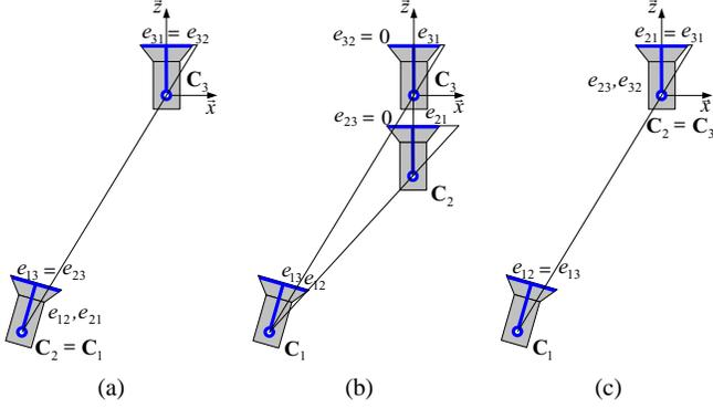
Fig. 3. Control strategy from the epipoles of three views. (a) Initial configuration. (b) Intermediate configuration. (c) Final configuration.
