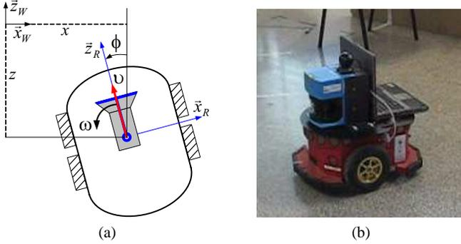
Fig. 1. Robotic system. (a) Frame definitions with  $\vec{x}_W, \vec{z}_W$  the axis of the world frame and  $\vec{x}_R, \vec{z}_R$  the corresponding for the robot frame. (b) Experimental platform.
