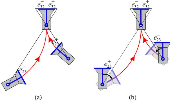
Fig. 4. Initial configurations requiring different motion strategy through adequate desired trajectories of the epipoles. (a)  $\text{sign}(e_{23}) \neq \text{sign}(e_{32})$  - direct motion toward the target. (b)  $\text{sign}(e_{23}) = \text{sign}(e_{32})$  - rotation to reach the same condition as in (a).
