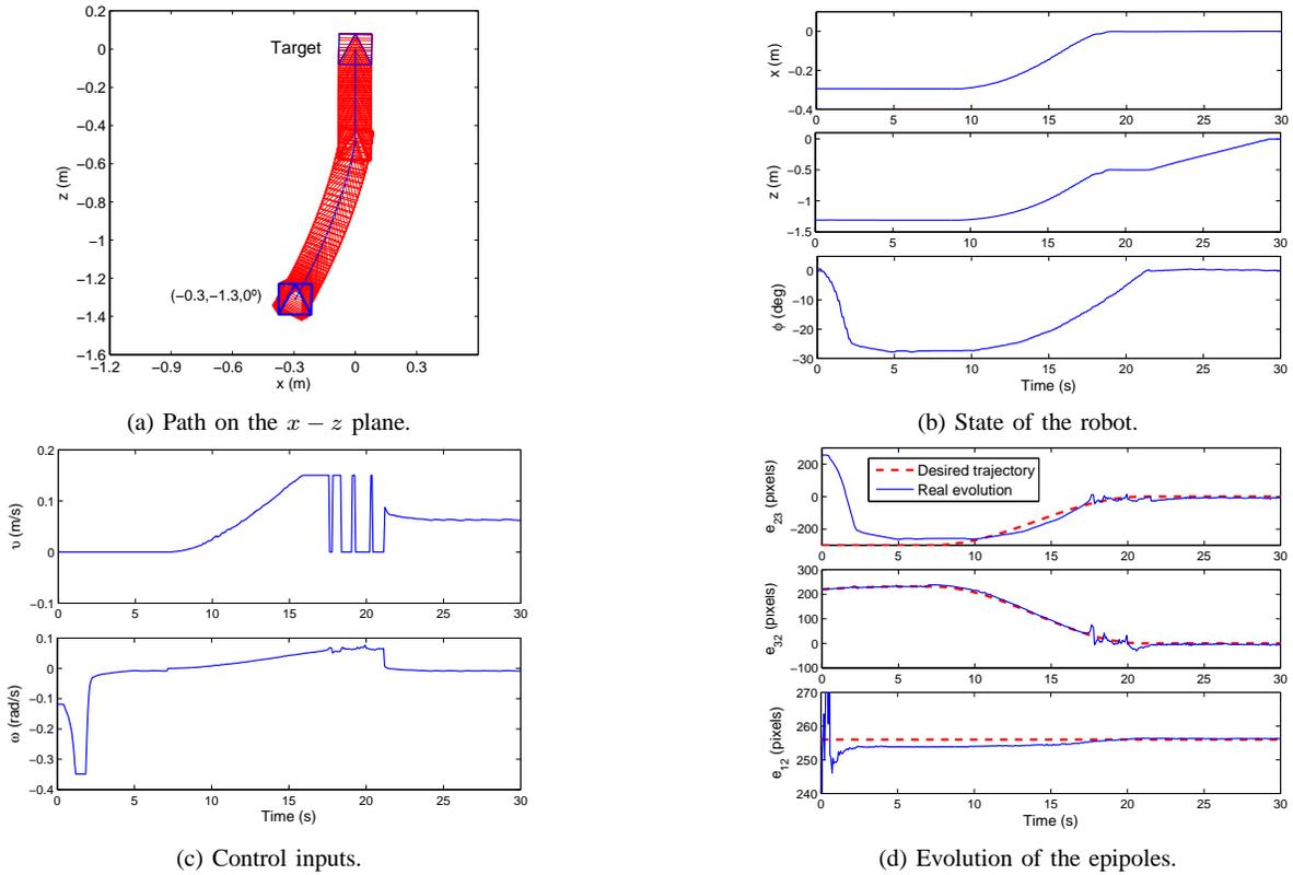
Fig. 9. Real experiment with target location  $(0,0,0^\circ)$ . The data presented in (a)-(b) corresponds to the robot odometry.
