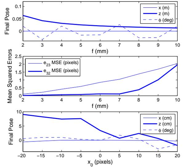
Fig. 7. Simulations with different values of focal length ( $f$ ) and principal point ( $x_0$ ) showing robustness against parametric uncertainty.
